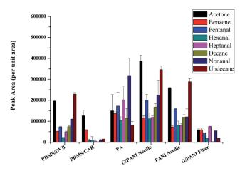
Fig. 4 Comparison with different commercial SPME fibers (PDMS/CAR, PDMS/DVB and PA), PANI needle and G/PANI fiber. VOCs concentration:  $2 \mu g L^{-1}$ .
