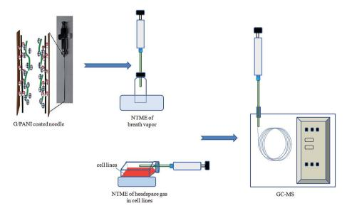
Fig. 1 Schematic diagram of NTME-GC-MS.
