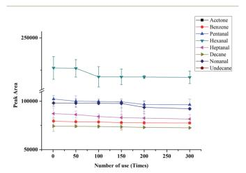
Fig. 3 Durability and lifetime of the coating. VOCs concentration: 2  $\mu$ g L<sup>-1</sup>.
