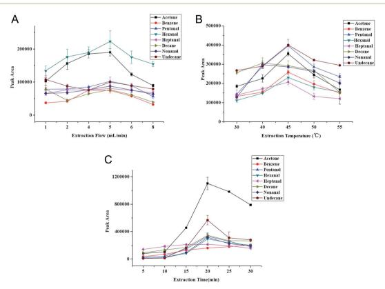
Selection of extraction conditions. (A) Sampling flow, (B) extraction temperature and (C) extraction time. VOCs concentration:  $2 \mu g L^{-1}$ .
