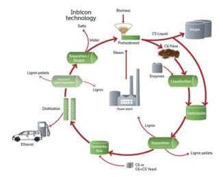
Fig. 1 The overall DONG Indicon technology process from where the liquid from hydrothermal pretreatment ("C5 liquid") was investigated.
