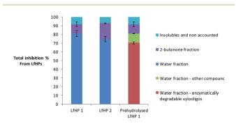
Fig. 5 Inhibition of cellulases exerted by the compounds in LfHP 1, LfHP 2 and LfHP 1 with enzymatic removal of xylooligosaccharides (prehydrolysed LfHP 1).
