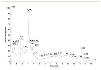
Fig. 6 Total ion chromatogram (negative ionisation) of pre-hydrolysed water fraction from 2-butanone extraction of LfHP 1. C2: compound 2 (Fig. 7), C3: compound 3 (Fig. 7), P<sub>3</sub>FA<sub>1</sub>: feruloylated tripentose, P<sub>3</sub>FA<sub>1</sub>Ac<sub>1</sub>: feruloylated acetylated tripentose.
