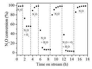
Fig. 8 Response of N<sub>2</sub>O conversion to step changes of co-feed 5% O<sub>2</sub> and/or 2% H<sub>2</sub>O over Rh/Zn-Al<sub>2</sub>O<sub>3</sub>-800 at 275 °C.
