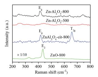
Fig. 3 Raman spectra for Zn-Al $_2$ O $_3$ -800, Zn-Al $_2$ O $_3$ -500, and ZnAl $_2$ O $_4$ -cit-800 (synthesized via citric acid route, pure ZnAl $_2$ O $_4$  phase) and ZnO-800 for comparison.
