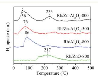
Fig. 10  $H_2$ -TPR profiles of Rh/Zn-Al<sub>2</sub>O<sub>3</sub>-800, Rh/Zn-Al<sub>2</sub>O<sub>3</sub>-500, Rh/Al<sub>2</sub>O<sub>3</sub>-800 and Rh/ZnO-800 catalysts.
