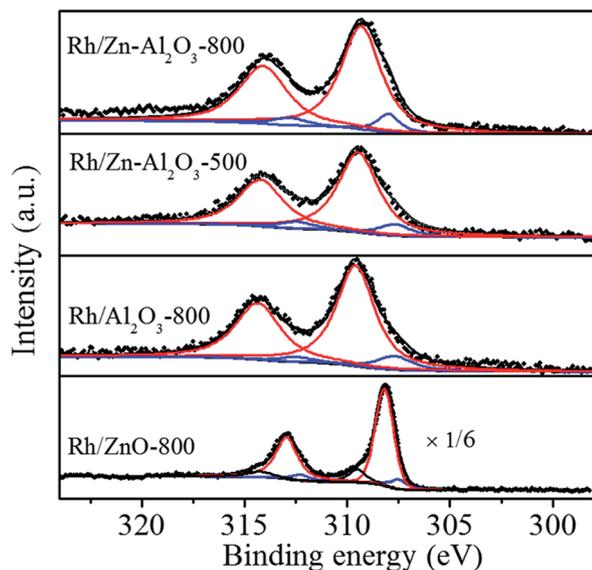
Fig. 5 Rh 3d XPS spectra of Rh/Zn-Al<sub>2</sub>O<sub>3</sub>-800, Rh/Zn-Al<sub>2</sub>O<sub>3</sub>-500, Rh/Al<sub>2</sub>O<sub>3</sub>-800, and Rh/ZnO-800.
