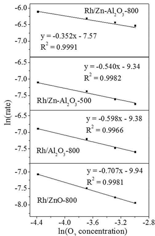
Fig. 9 Influence of O<sub>2</sub> concentration on the activities of Rh/Zn-Al<sub>2</sub>O<sub>3</sub>-800, Rh/Zn-Al<sub>2</sub>O<sub>3</sub>-500, Rh/Al<sub>2</sub>O<sub>3</sub>-800, and Rh/ZnO-800 in N<sub>2</sub>O decomposition.
