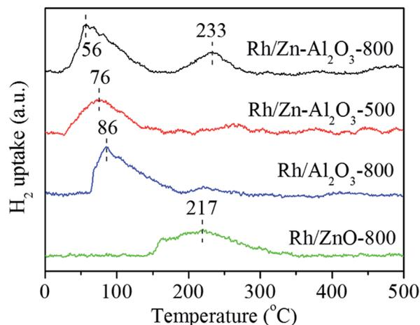
Fig. 10 H<sub>2</sub>-TPR profiles of Rh/Zn-Al<sub>2</sub>O<sub>3</sub>-800, Rh/Zn-Al<sub>2</sub>O<sub>3</sub>-500, Rh/Al<sub>2</sub>O<sub>3</sub>-800 and Rh/ZnO-800 catalysts.
