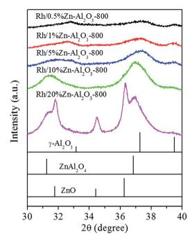
Fig. 2 XRD patterns of Rh/Zn–Al $_2O_3$ -800 catalysts with different Zn loading and standard patterns of  $\gamma$ -Al $_2O_3$  (PDF#47-1308), ZnAl $_2O_4$  (PDF#05-0699), and ZnO (PDF#36-1451).
