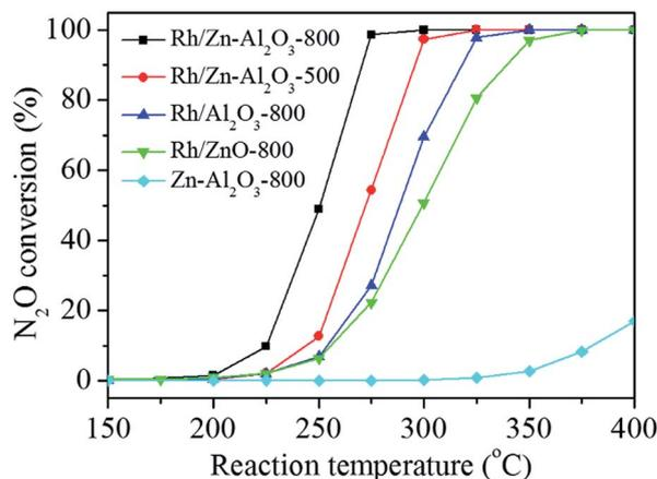
Fig. 6 Conversion of N<sub>2</sub>O on the catalysts as a function of reaction temperature.
