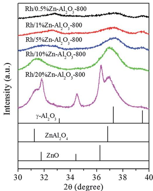
Fig. 2 XRD patterns of Rh/Zn- $\text{Al}_2\text{O}_3$ -800 catalysts with different Zn loading and standard patterns of  $\gamma$ - $\text{Al}_2\text{O}_3$  (PDF#47-1308),  $\text{ZnAl}_2\text{O}_4$  (PDF#05-0699), and ZnO (PDF#36-1451).
