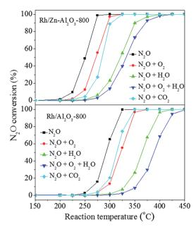
Fig. 7 Influence of co-feed 5% O2, 2% H2O, or 2% CO2 on the conversion of N<sub>2</sub>O over Rh/Zn-Al<sub>2</sub>O<sub>3</sub>-800 and Rh/Al<sub>2</sub>O<sub>3</sub>-800 as a function of reaction temperature.
