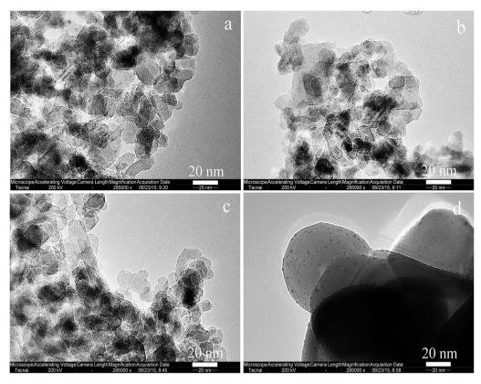
Fig. 4 TEM graphs of (a) Rh/Zn-Al<sub>2</sub>O<sub>3</sub>-800, (b) Rh/Zn-Al<sub>2</sub>O<sub>3</sub>-500, (c) Rh/Al<sub>2</sub>O<sub>3</sub>-800, and (d) Rh/ZnO-800.
