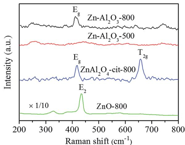
Fig. 3 Raman spectra for Zn- $\text{Al}_2\text{O}_3$ -800, Zn- $\text{Al}_2\text{O}_3$ -500, and  $\text{ZnAl}_2\text{O}_4$ -cit-800 (synthesized *via* citric acid route, pure  $\text{ZnAl}_2\text{O}_4$  phase) and ZnO-800 for comparison.
