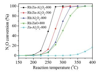
Fig. 6 Conversion of  $\ensuremath{\text{N}}_2\ensuremath{\text{O}}$  on the catalysts as a function of reaction temperature.
