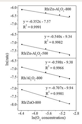
Fig. 9 Influence of O2 concentration on the activities of Rh/Zn- $Al_2O_3$ -800,  $Rh/Zn-Al_2O_3$ -500,  $Rh/Al_2O_3$ -800, and Rh/ZnO-800 in N<sub>2</sub>O decomposition.
