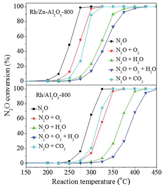
Fig. 7 Influence of co-feed 5% O<sub>2</sub>, 2% H<sub>2</sub>O, or 2% CO<sub>2</sub> on the conversion of N<sub>2</sub>O over Rh/Zn-Al<sub>2</sub>O<sub>3</sub>-800 and Rh/Al<sub>2</sub>O<sub>3</sub>-800 as a function of reaction temperature.
