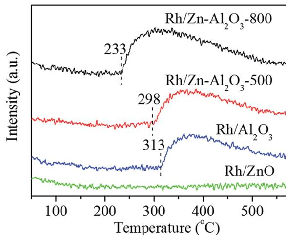
Fig. 11 O<sub>2</sub>-TPD profiles of Rh/Zn-Al<sub>2</sub>O<sub>3</sub>-800, Rh/Zn-Al<sub>2</sub>O<sub>3</sub>-500, Rh/Al<sub>2</sub>O<sub>3</sub>-800 and Rh/ZnO-800 catalysts.
