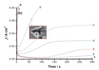
Fig. 2 Chronoamperometry measurements recorded for (a) alloy I (CoNiGa SMA) and (b) alloy II (CoNiGaAl SMA) in 0.5 M NaCl solutions at 25 °C as a function of the applied anodic potential ( $E_a$ ). (1) -0.2 V(SCE); (2) -0.1 V(SCE); (3) 0.0 V(SCE); (4) +0.1 V(SCE); (5) +0.2 V(SCE); (6) +0.3 V(SCE); (7) +0.4 V(SCE); (8) +0.5 V(SCE). Insets: SEM images captured for the two alloys in 0.5 M NaCl solutions at 25 °C after holding the alloy at  $E_a = 0.3$  V(SCE) for 60 s.
