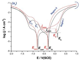
Fig. 1 Cyclic polarization curves (upper) linear and (lower) logarithmic scales recorded for CoNiGa (alloy I) and CiNiGaAl (alloy II) in 0.5 M NaCl solution at 25 °C. Measurements were conducted between -2.0 V(SCE) and +1.0 V(SCE) at a scan rate of 5.0 mV s $^{-1}$ .
