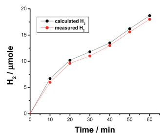
Fig. 5 Volume of  $H_2$  calculated from the amount of charge passed (assuming 100% faradaic efficiency) and that of  $H_2$  measured from gas chromatography during 1 h of a controlled potential electrolysis run of the best catalyst (the pitted surface of alloy II) at -0.8 V vs. RHE in 0.1 M KOH aqueous solution.
