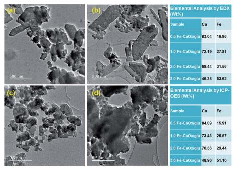
Fig. 5 TEM micrographs of (a) 0.5 Fe-CaOx/glu (b) 1.0 Fe-CaOx/glu (c) 2.0 Fe-CaOx/glu (d) 3.0 Fe-CaOx/glu; elemental analysis by EDX and ICP-OES.
