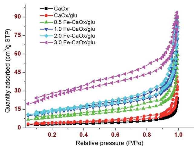
Fig. 7 N<sub>2</sub> adsorption/desorption isotherms at 77 K.
