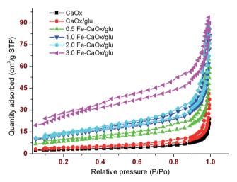
Fig. 7 N<sub>2</sub> adsorption/desorption isotherms at 77 K.
