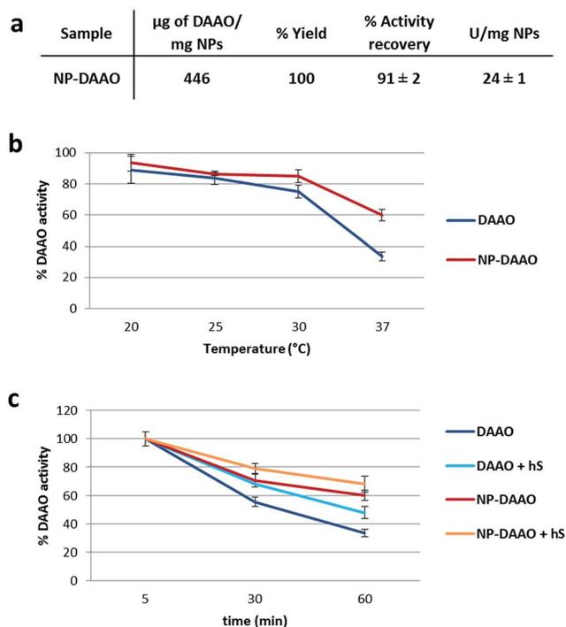
**Fig. 3** (a) NP-DAAO system features; U are enzymatic units of DAAO. (b) Thermal stability, measured as enzymatic activity, of the NP-DAAO system after 1 h incubation; (c) effect of 10% human serum (hS) on NP-DAAO during 1 h incubation. Error bars represent mean  $\pm$  SD,  $N = 3$ .
