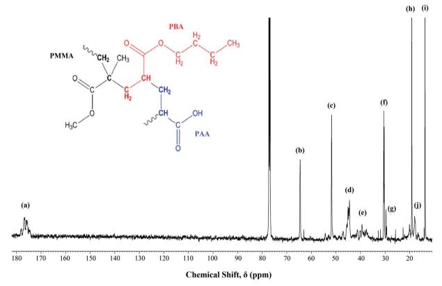
Fig. 1 <sup>13</sup>C NMR of UHMW-P(MMA-co-BA-co-AA) thin film measured at room temperature. Inset: copolymer structure.
