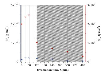
Fig. 6 Changes in average-molecular weights at different UV irradiation time. Note: blue and red color symbols/Y-axis are respectively represent  $M_n$  and  $M_w$  values. Symbols representation; star: non-irradiated sample, down-pointing triangle and circle: irradiated samples (open symbol-cross linked structure and filled symbol-fragmentation). Dense region showed degraded samples.
