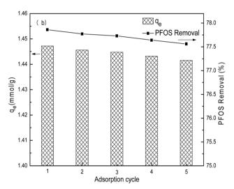
Fig. 15 Desorption of spent PACFs using different regeneration agents (a), and sorption of PFOS on the PACFs in five sorption cycles (b).
