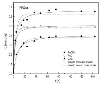
Fig. 6 Sorption kinetics of PFOS and PFOA on the PACFs, PAC and GAC respectively, fitted with pseudo-first-order and pseudo-second-order kinetics models.
