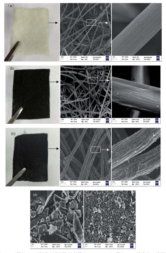
Fig. 1 Digital photos and SEM images of PANFs (a), PANOFs (b), PACFs (c), compared to the SEM images of PAC (d) and GAC (e).
