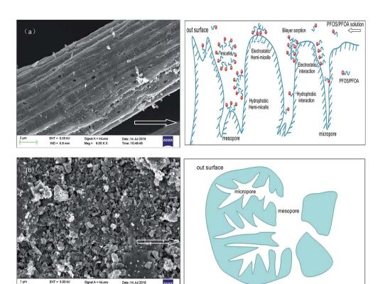
Fig. 13 Schematic diagram for the sorption of PFOS and PFOA on the positively charged PANF-derived PACFs (a), and schematic view of the pore structure of GAC (b).
