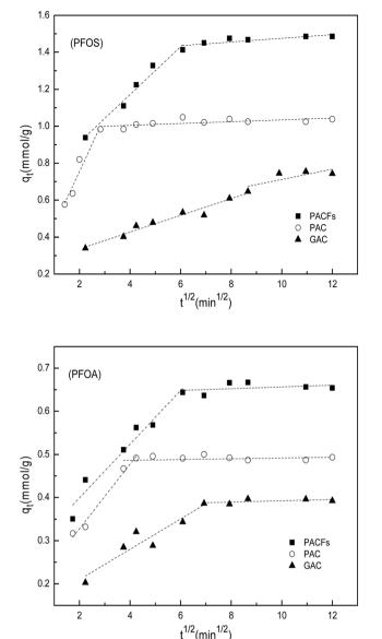
Fig. 7 Intra-particle diffusion model for the sorption of PFOS and PFOA on the PACFs, PAC and GAC.
