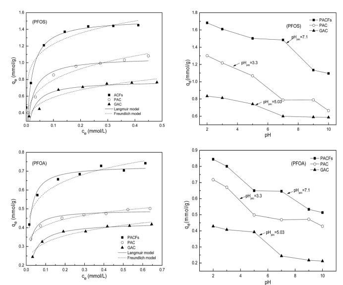
Fig. 9 Sorption isotherms of PFOS and PFOA on the PACFs, PAC and GAC respectively, fitted with Langmuir model and Freundlich model.
