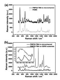
Fig. 8 (a) SERS signals of PMP22-TM4 in microchannel and PDMS control experiment; (b) the SERS signals of PMP22-TM4 in microchannel and on SERS substrate. The concentration of PMP22-TM4 was 3.6  $\mu$ M and the buffer condition was 0.2 M acetate buffer at pH 5.5, 0.5% DPC and 150 mM NaCl. The flow rate was 0.11 cm s<sup>-1</sup>.
