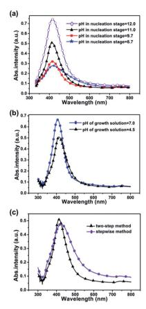
Fig. 2 (a) UV-visible extinction spectra of the silver colloids nucleating at various pH values (8.7, 9.7, 11.0 and 12.0) and growing at pH 5; (b) UV-visible extinction spectra of the silver colloids growing at pH 7.4 and pH 5 (corresponding pH values of growth solutions were 7.0 and 4.5), while nucleating at pH 11.0; (c) UV-visible extinction spectra of silver colloids prepared by two-step method and stepwise method (the pH values in nucleation are 11; the pH values in growth are 5).
