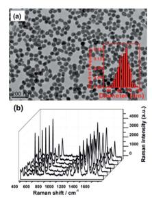
Fig. 3 (a) The TEM image of finally prepared Ag NPs; (b) SERS spectra of R6G in silver colloids detected at 6 random spots. (The experiment was done by mixing 100  $\mu$ l R6G (10 $^{-3}$  M) in 900  $\mu$ l silver colloids (approximately 160  $\mu$ M), then collected SERS signals at six random spots of the mixture solution. The resulting concentration of R6G was  $10^{-4} M.$
