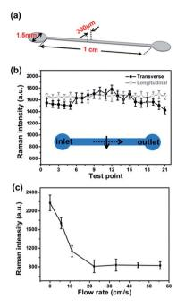
Fig. 7 (a) The structure and sizes of the microchannel. The depth is 50  $\mu$ m; (b) transverse and longitudinal measurements, flow rate was set to 5.6 cm s<sup>-1</sup>; (c) the relationship between SERS intensity and flow rate. SERS intensities at 1510 cm<sup>-1</sup> band of R6G (1  $\mu$ M) are shown in the figure. Each point is the average of 6 measurements and error bar is the RSD; the integral time was 3 s; the interval of each detection spot was 10  $\mu$ m.
