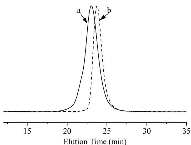
Fig. 4 GPC traces of copolymers: (a) PS-*b*-PI-*b*-PMMA; (b) PS-*b*-PI.
