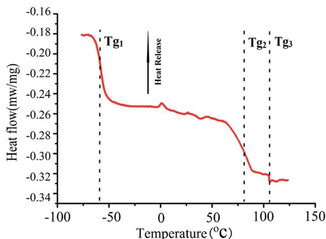
Fig. 7 DSC curves of PS-*b*-PI-*b*-PMMA.
