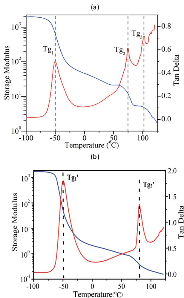
Fig. 6 Dynamic mechanical curves of PS-*b*-PI-*b*-PMMA (a) and PS-*b*-PI (b).
