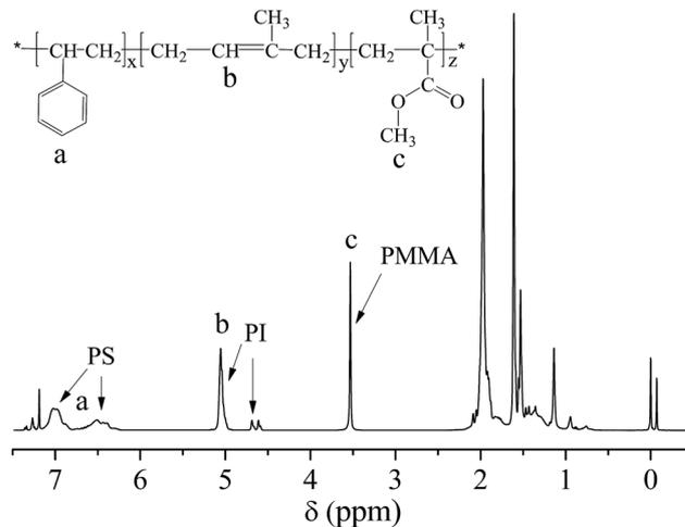
Fig. 5 <sup>1</sup>H-NMR spectrum of PS-*b*-PI-*b*-PMMA.
