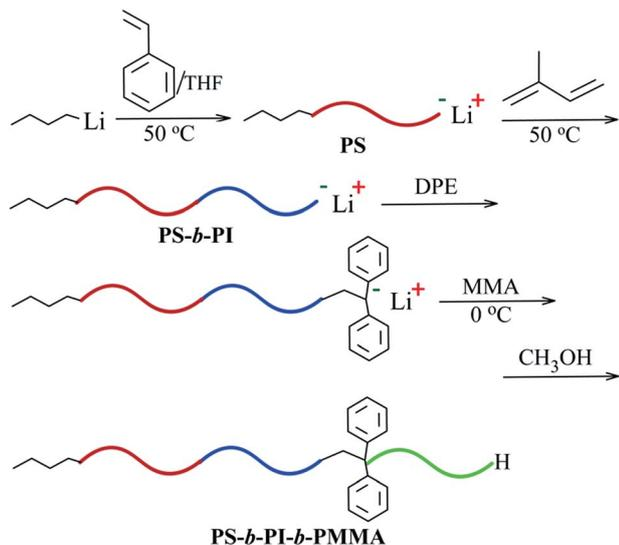
Scheme 1 Synthesis mechanism of PS-*b*-PI-*b*-PMMA.
