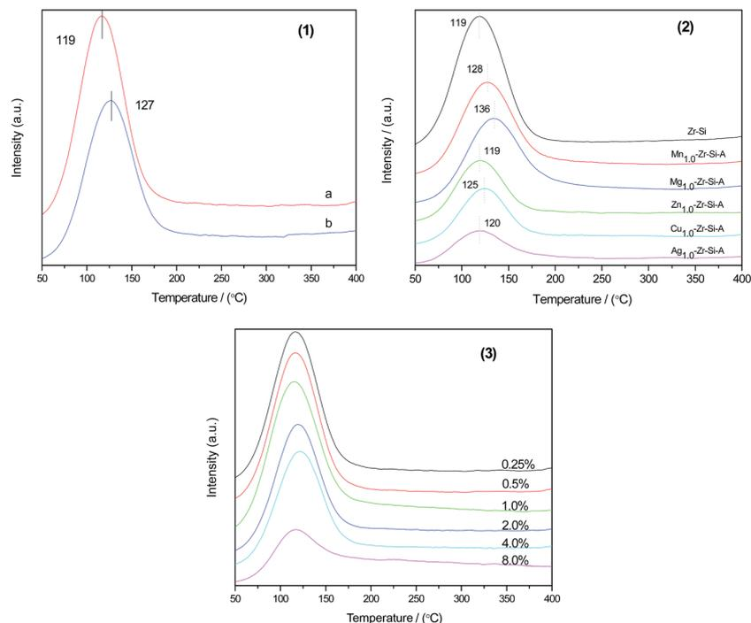
Fig. 5  $\text{NH}_3$ -TPD profiles of (1) Zn-Zr-Si catalysts prepared by two different methods: (a)  $\text{Zn}_{1.0}$ -Zr-Si-A; (b)  $\text{Zn}_{1.0}$ -Zr-Si-B; (2) different metal oxide promoted Zr-Si catalysts; (3) Zn-Zr-Si-A catalyst samples with different ZnO contents.
