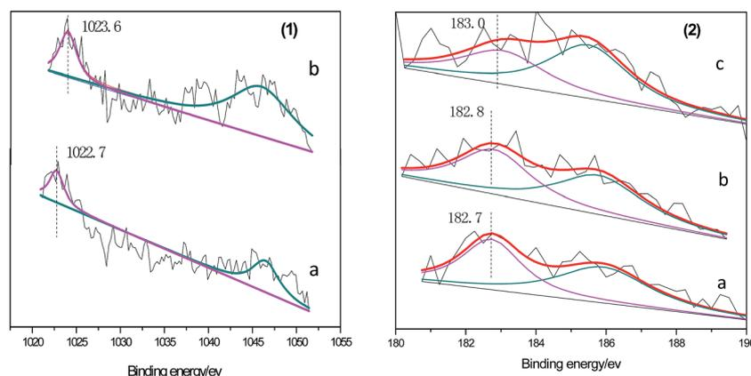
Fig. 4 (1) XPS profiles of  $\text{Zn 2p}$  (a)  $\text{Zn}_{1.0}\text{-Zr-Si-B}$ ; (b)  $\text{Zn}_{1.0}\text{-Zr-Si-A}$ ; (2) XPS profiles of  $\text{Zr 3d}$  for: (a)  $\text{Zr-Si}$ ; (b)  $\text{Zn}_{1.0}\text{-Zr-Si-B}$ ; (c)  $\text{Zn}_{1.0}\text{-Zr-Si-A}$ .
