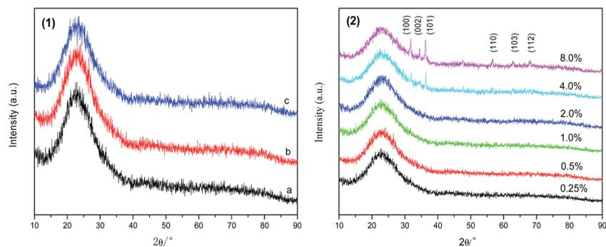
Fig. 1 XRD patterns for the catalysts (1) catalyst samples prepared by different method (a) Zr-Si; (b) Zn<sub>1.0</sub>-Zr-Si-A; (c) Zn<sub>1.0</sub>-Zr-Si-B; (2) catalyst samples with different ZnO contents.
