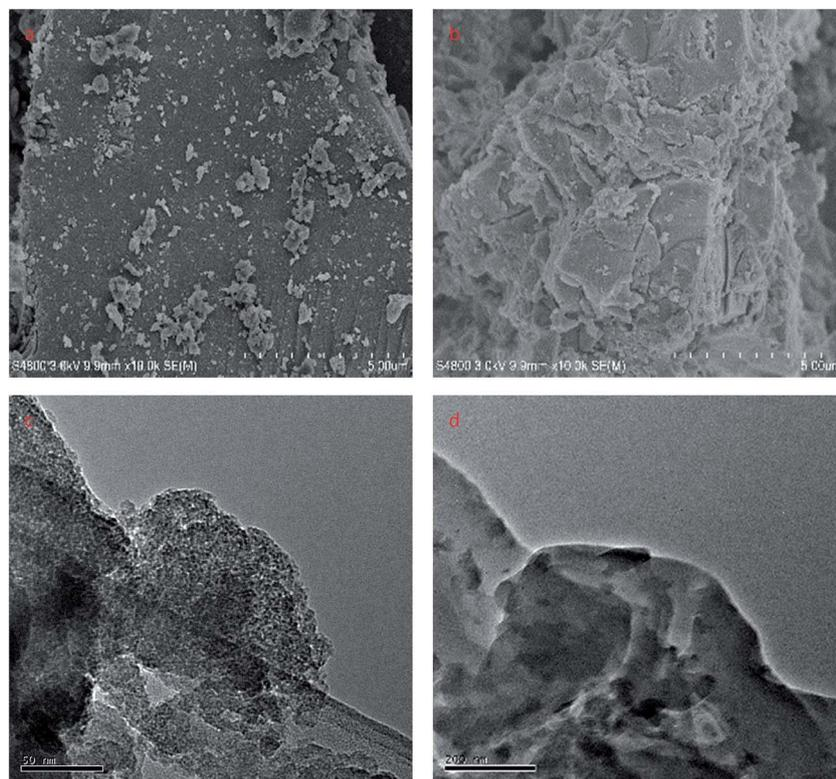
Fig. 2 SEM image (5 μm) of (a) Zn<sub>1.0</sub>-Zr-Si-A, (b) Zn<sub>1.0</sub>-Zr-Si-B. TEM image of (c) Zn<sub>1.0</sub>-Zr-Si-A (50 nm), (d) Zn<sub>1.0</sub>-Zr-Si-B (200 nm).
