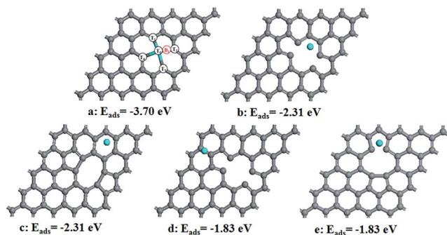
Fig. 1 (a–e) Configurations refer to possible adsorption sites for Sn atom at a divacancy in graphene.  $E_{\text{ads}}$  refers to the corresponding adsorption energy.  $T_0$ ,  $T_1$ ,  $T_2$ ,  $T_3$  and  $T_4$  in a configuration refer to the top sites, while  $B_1$  refers to the bridge site between Sn and C atoms. The gray and blue balls represent C and Sn atoms, respectively.
