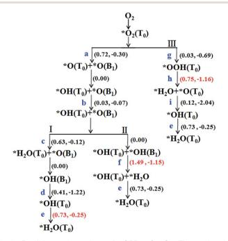
Fig. 3 Possible reaction pathways for ORR on Sn-Gra. The numbers in parenthesis are the energy barriers (left) and reaction energies (right) in units of eV. For the details of labels (a-i) see Fig. 4. \* denotes that the ORR species is adsorbed on the catalyst surface.
