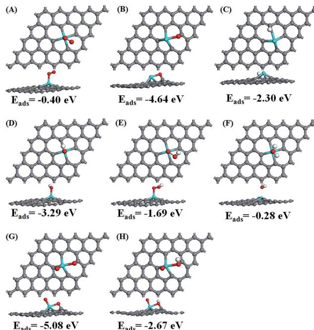
Fig. 2 Atomic structures with the lowest adsorption energy for the ORR species (the second lowest adsorption energy for H atom) adsorbed on Sn–Gra. (A)  $\text{O}_2$ , (B) O, (C) H, (D) OH, (E) OOH, (F)  $\text{H}_2\text{O}$ , (G) two separated O atoms; (H) O + OH.  $E_{\text{ads}}$  represents the adsorption energy.
