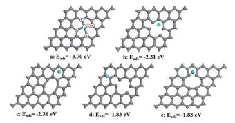
Fig. 1 (a–e) Configurations refer to possible adsorption sites for Sn atom at a divacancy in graphene.  $E_{\rm ads}$  refers to the corresponding adsorption energy.  $T_0$ ,  $T_1$ ,  $T_2$ ,  $T_3$  and  $T_4$  in a configuration refer to the top sites, while  $B_1$  refers to the bridge site between Sn and C atoms. The gray and blue balls represent C and Sn atoms, respectively.
