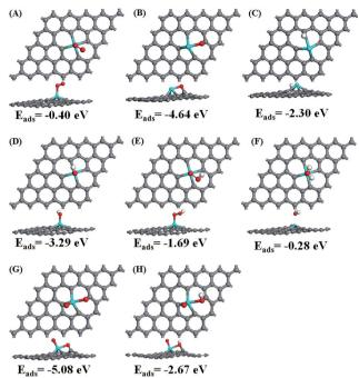
Fig. 2 Atomic structures with the lowest adsorption energy for the ORR species (the second lowest adsorption energy for H atom) adsorbed on Sn–Gra. (A) O<sub>2</sub>, (B) O, (C) H, (D) OH, (E) OOH, (F) H<sub>2</sub>O, (G) two separated O atoms; (H) O + OH.  $E_{\rm ads}$  represents the absorption energy.
