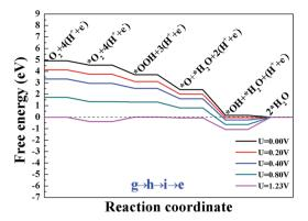
Fig. 5 The free energy diagram for the most favorite reaction pathway III (g  $\rightarrow$  h  $\rightarrow$  i  $\rightarrow$  e) on Sn–Gra at different electrode potentials.
