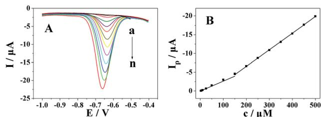
Fig. 9 (A) DPVs of metronidazole at the Pt nanospheres/polyfurfural film/GCE in BR (pH 10) buffer solution. Concentrations: 2.5, 5, 10, 25, 50, 100, 150, 200, 250, 300, 350, 400, 450 and 500  $\mu\text{mol dm}^{-3}$  (from a to n). (B) Linear relationship between reduction peak current and concentration.
