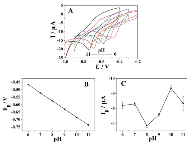
Fig. 8 CVs of (A) metronidazole ( $200 \mu\text{mol dm}^{-3}$ ) in BR buffer solution at different pH values on the Pt nanospheres/polyfurfural film/GCE. The relationship of (B) pH vs. reduction peak potential and (C) pH vs. reduction peak current ( $I_p$ ) for metronidazole ( $n = 3$ ).
