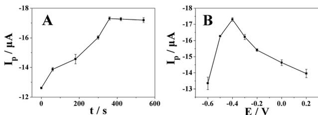
Fig. 7 The effect of accumulation time (A) and accumulation potential (B) on the reduction peak current of  $500 \mu\text{mol dm}^{-3}$  metronidazole in BR (pH 10) buffer solution at the Pt nanospheres/polyfurfural film/GCE ( $n = 3$ ).
