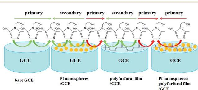
Fig. 4 The electrocatalytic reaction mechanisms of metronidazole.
