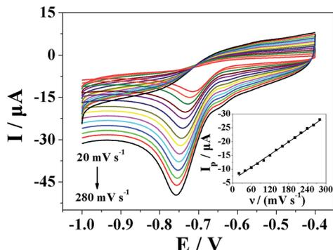
Fig. 6 CVs of metronidazole ( $500 \mu\text{mol dm}^{-3}$ ) at the Pt nanospheres/polyfurfural film/GCE in BR (pH 10) buffer solution at different scan rates (20, 40, 60, 80, 100, 120, 140, 160, 180, 200, 220, 240, 260,  $280 \text{ mV s}^{-1}$ ). Inset: the relationship between the reduction peak current and scan rate.
