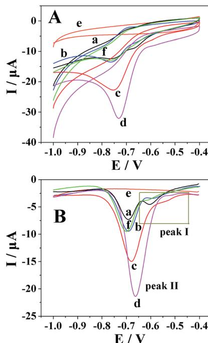
Fig. 3 CVs (A) and DPVs (B) of  $500 \mu\text{mol dm}^{-3}$  metronidazole in BR (pH 10) buffer solution at (a) bare GCE, (b) Pt nanospheres/GCE, (f) bare platinum electrode, (c) polyfurfural film/GCE and (d) Pt nanospheres/polyfurfural film/GCE. CVs (A) and DPVs (B) of Pt nanospheres/polyfurfural film/GCE in BR (pH 10) buffer solution without metronidazole (e).
