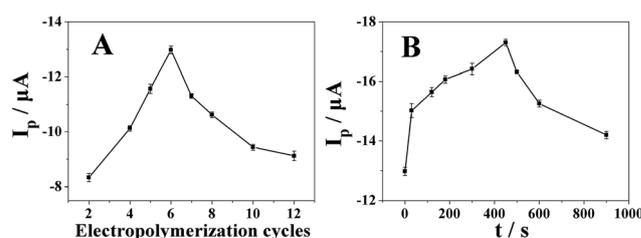
Fig. 5 The effect of (A) electropolymerization cycles of furfural and (B) deposit time of platinum on the reduction peak current of  $500 \mu\text{mol dm}^{-3}$  metronidazole in BR (pH 10) buffer solution ( $n = 3$ ).
