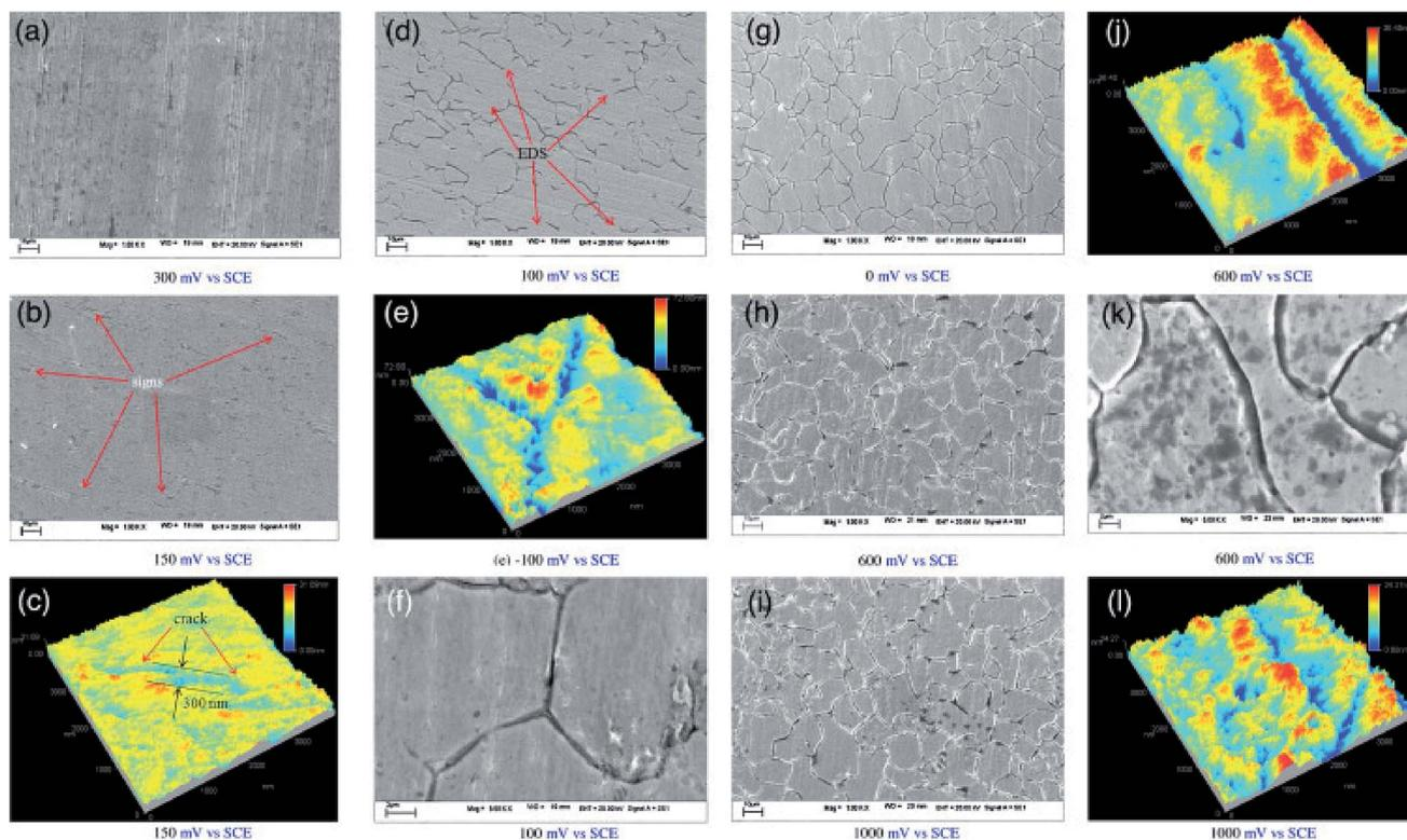
Fig. 18 SEM morphologies and STM topographies of mild steel polarized at (a)  $-300$  mV vs. SCE, (b)  $-150$  mV vs. SCE, (c)  $-150$  mV vs. SCE, (d)  $100$  mV vs. SCE, (e)  $-100$  mV vs. SCE, (f)  $-100$  mV vs. SCE, (g)  $0$  mV vs. SCE, (h)  $600$  mV vs. SCE, (i)  $1000$  mV vs. SCE, (j)  $600$  mV vs. SCE, (k)  $600$  mV vs. SCE, (l)  $1000$  mV vs. SCE (in  $\text{CO}_2 + \text{NaNO}_2$  solution).<sup>159</sup> Reprinted with permission from ref. 159. Copyright 2015, Elsevier B. V.
