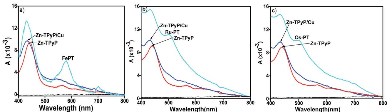
Fig. 3 UV-vis spectra of Cu<sup>2+</sup>-mediated molecular dyads for (a) Zn-TPyP/Cu/Fe-PT, (b) Zn-TPyP/Cu/Ru-PT, and (c) Zn-TPyP/Cu/Os-PT layers fabricated on glass substrates. Solid black, red, blue, and cyan lines represent the corresponding spectrum of the glass baseline, Zn-TPyP monolayers, Cu-terminated monolayers and the respective dyad layers.
