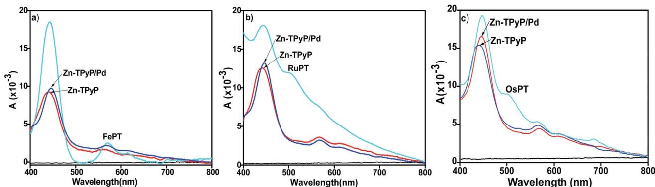
Fig. 4 UV-vis spectra of  $\text{Pd}^{2+}$ -mediated molecular dyads for (a) Zn-TPyP/Pd/Fe-PT, (b) Zn-TPyP/Pd/Ru-PT, and (c) Zn-TPyP/Pd/Os-PT layers prepared on the glass substrates. Solid black, red, blue, and cyan lines represent the corresponding spectrum of the glass baseline, Zn-TPyP monolayers, Pd-terminated monolayers and the respective dyad layers.
