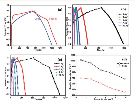
Fig. 5 (a) Galvanostatic charge-discharge of CoSe and CoSe-G at a constant current density of 1 A g<sup>-1</sup>; (b) galvanostatic charge-discharge studies of CoSe at different current densities; (c) galvanostatic charge-discharge studies of CoSe-G at different current densities; (d) specific capacitance of CoSe and CoSe-G electrodes as a function of different current densities.
