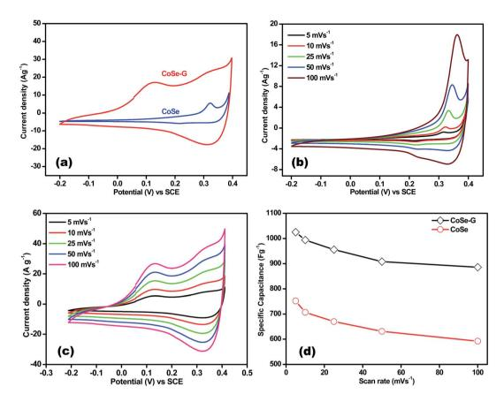
Fig. 4 (a) Cyclic voltammograms of CoSe and CoSe–G at 25 mV s<sup>-1</sup>; (b) cyclic voltammograms of CoSe at different scan rates; (c) cyclic voltammograms of CoSe–G at different scan rates; (d) specific capacitance of CoSe and CoSe–G electrodes as a function of different scan rates.
