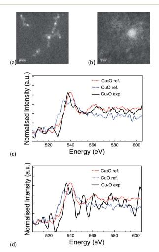
Fig. 5 (a) & (b) STEM image of PVP capped copper oxide NMs, (c) spectrum showing similarity to the O K-edge of  $Cu_2O$  & (d) spectrum showing no similarity to  $Cu_2O$  or CuO reference NMs.
