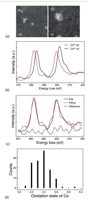
Fig. 6 (a) STEM images for 10k PVP capped ceria, (b) reference EELS spectra of commercially available  $Ce^{3+}$  ( $Ce(NO_3)_3$  salt); and  $Ce^{4+}$  ( $CeO_2$  NMs) materials; (c) MLLS fitting of an EELS spectrum from one  $CeO_x$  NM; & (d) oxidation state distribution of  $CeO_x$  NPs.
