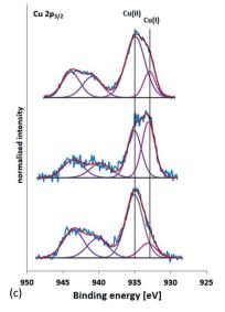
Fig. 4 (a) XPS spectra of 10k PVP capped ceria NMs, 40k PVP capped ceria NMs and 360k PVP capped ceria from bottom to top respectively. The peak at 916.7 eV is a characteristic satellite peak indicating the presence of cerium(iv). (b) Zn  $2p_{3/2}$  XPS spectrum for 10, 40 and 360k PVP capped zinc oxide NM samples. (c) Cu  $2p_{3/2}$  XPS spectra for 10, 40 and 360k PVP capped copper oxide NMs (bottom to top) indicating the presence of both copper(ii) and copper(i) species.
