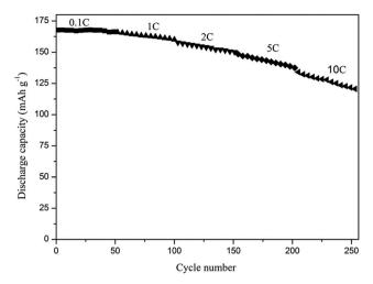
Fig. 10 The cycle performance of cell with 2% in situ  $SiO_2$  at different current rates (1C = 170 mA h  $g^{-1}$ ).
