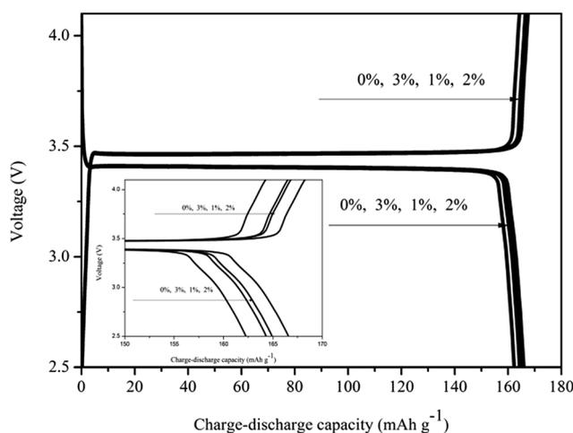
Fig. 9 First charge–discharge capacities of GPEs based on electrospun membrane with and without *in situ* SiO<sub>2</sub>.
