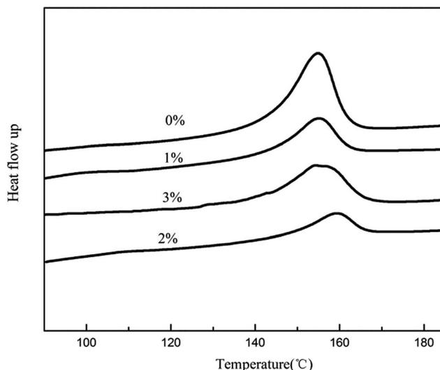
Fig. 4 DSC curves of the electrospun PVDF-HFP/TPU/PMMA membranes with and without *in situ* SiO<sub>2</sub>.
