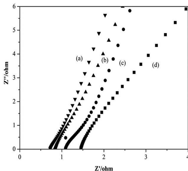
Fig. 6 Impedance spectra of gel polymer electrolytes (a) with 2% *in situ* SiO<sub>2</sub> (b) with 1% *in situ* SiO<sub>2</sub> (c) with 3% *in situ* SiO<sub>2</sub> (d) without *in situ* SiO<sub>2</sub>.
