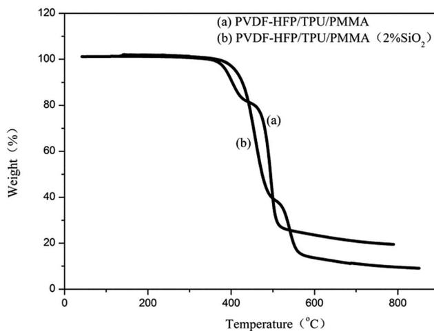
Fig. 3 Thermograms of electrospun PVDF-HFP/TPU/PMMA membranes (a) without *in situ* SiO<sub>2</sub> (b) with 2% *in situ* SiO<sub>2</sub>.
