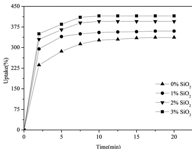
Fig. 5 The uptake behavior of electrospun PVDF–HFP/TPU/PMMA membranes with and without *in situ* SiO<sub>2</sub>.
