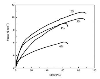
Fig. 8 Stress-strain curves of electrospun PVDF-HFP/TPU/PMMA membranes with and without *in situ* SiO<sub>2</sub>.
