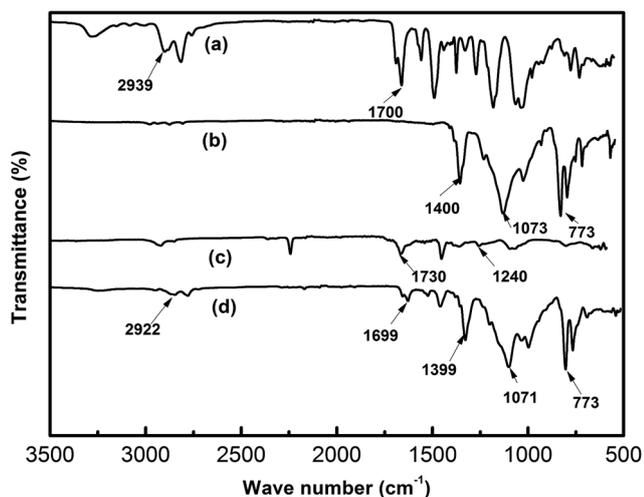
Fig. 2 FTIR spectra of the electrospun membranes (a) TPU (b) PVDF-HFP (c) PMMA (d) PVDF-HFP/TPU/PMMA membranes with *in situ* SiO<sub>2</sub>.
