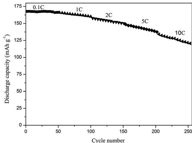
Fig. 10 The cycle performance of cell with 2% *in situ* SiO<sub>2</sub> at different current rates (1C = 170 mA h g<sup>-1</sup>).
