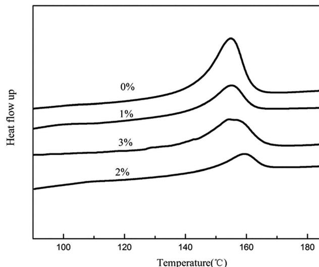
Fig. 4 DSC curves of the electrospun PVDF-HFP/TPU/PMMA membranes with and without *in situ* SiO<sub>2</sub>.
