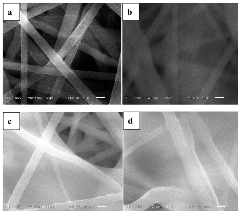
Fig. 1 SEM images of electrospun PVDF–HFP/TPU/PMMA membranes (a) without *in situ* SiO<sub>2</sub> (b) with 1% *in situ* SiO<sub>2</sub> (c) with 2% *in situ* SiO<sub>2</sub> (d) with 3% *in situ* SiO<sub>2</sub>.
