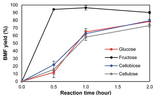
Fig. 4 Conversion of different carbohydrates into BMF. Note: reaction conditions: 2% (w/v) (200 mg) of carbohydrates loading with 0.16 M of HBr in 10 mL of LiBr hydrate (61.6%), 20 mL of organic phase (DCM), 125 °C, 500 rpm for stirring, 0–120 min.
