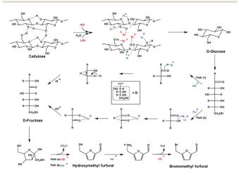
Fig. 5 Proposed conversion pathways from cellulose to BMF.
