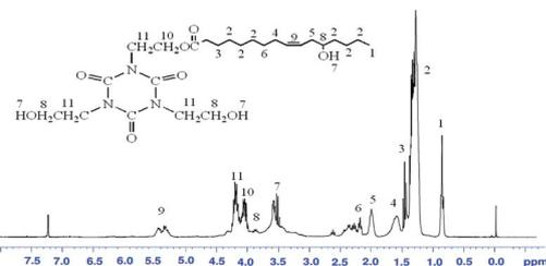
Fig. 4  $^1\text{H}$  NMR spectrum of THEIC-MR.
