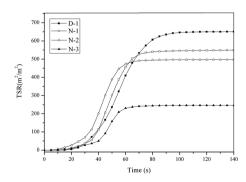
Fig. 12 TSR curves of PVC blends.
