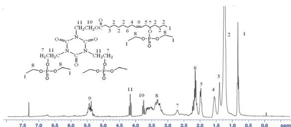
Fig. 5  $^1\text{H}$  NMR spectrum of THEIC-MR-phosphate.
