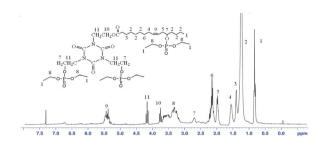
Fig. 5 <sup>1</sup>H NMR spectrum of THEIC-MR-phosphate.
