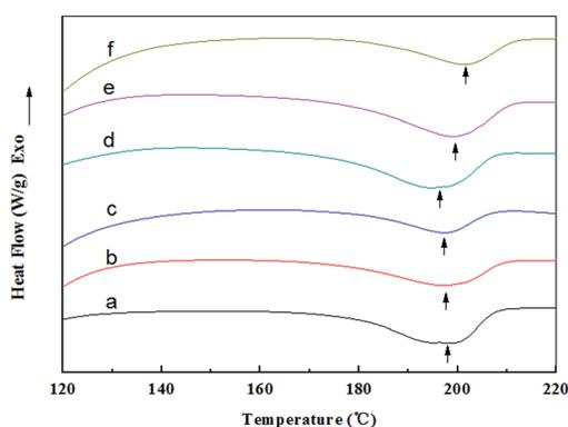
Fig. 8 DSC curves of random and aligned nanofibers: (a) RNFs-FK<sub>0</sub>PVA<sub>10</sub>, (b) RNFs-FK<sub>1</sub>PVA<sub>9</sub>, (c) RNFs-FK<sub>4</sub>PVA<sub>6</sub>, (d) ANFs-FK<sub>0</sub>PVA<sub>10</sub>, (e) ANFs-FK<sub>1</sub>PVA<sub>9</sub>, (f) ANFs-FK<sub>4</sub>PVA<sub>6</sub>.
