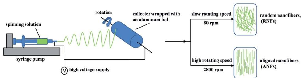
Fig. 1 Schematic representation of the applied electrospinning process.
