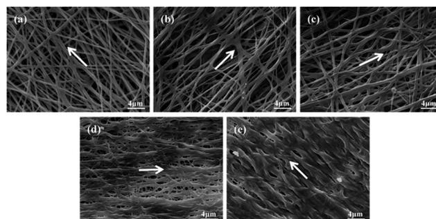
Fig. 5 SEM images of electrospun aligned nanofibers (ANFs) with various blending ratios: (a) FK<sub>0</sub>PVA<sub>10</sub>, (b) FK<sub>1</sub>PVA<sub>9</sub>, (c) FK<sub>2</sub>PVA<sub>8</sub>, (d) FK<sub>3</sub>PVA<sub>7</sub>, (e) FK<sub>4</sub>PVA<sub>6</sub>. Notes: the white arrow indicates the orientation of the ANFs.
