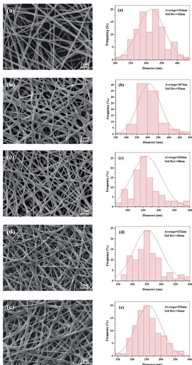
Fig. 4 SEM images and diameter distributions of electrospun random nanofibers (RNFs) with various blending ratios: (a) FK<sub>0</sub>PVA<sub>10</sub>, (b) FK<sub>1</sub>PVA<sub>9</sub>, (c) FK<sub>2</sub>PVA<sub>8</sub>, (d) FK<sub>3</sub>PVA<sub>7</sub>, (e) FK<sub>4</sub>PVA<sub>6</sub>.
