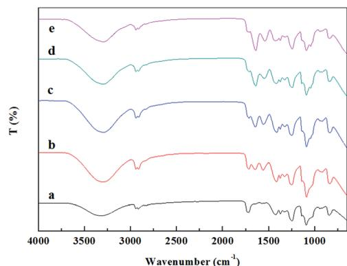
Fig. 6 FTIR spectra of the RNFs with various blending ratios: (a) RNFs–FK<sub>0</sub>PVA<sub>10</sub>, (b) RNFs–FK<sub>1</sub>PVA<sub>9</sub>, (c) RNFs–FK<sub>2</sub>PVA<sub>8</sub>, (d) RNFs–FK<sub>3</sub>PVA<sub>7</sub>, (e) RNFs–FK<sub>4</sub>PVA<sub>6</sub>.
