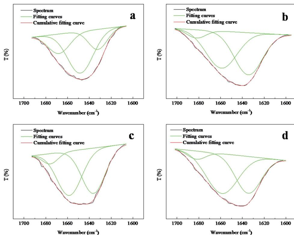
Fig. 7 Amide I region spectra of random and aligned nanofibers: (a) RNFs–FK<sub>1</sub>PVA<sub>9</sub>, (b) RNFs–FK<sub>4</sub>PVA<sub>6</sub>, (c) ANFs–FK<sub>1</sub>PVA<sub>9</sub>, (d) ANFs–FK<sub>4</sub>PVA<sub>6</sub>.
