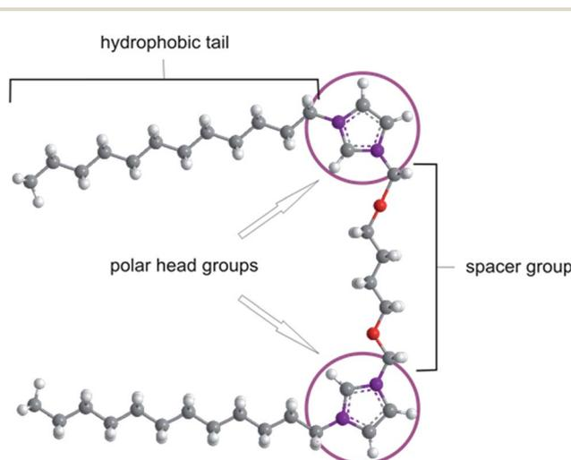
Fig. 1 Generic structure of a gemini surfactant.
