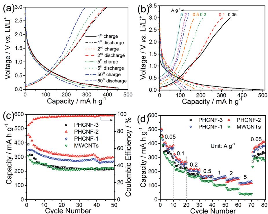
Fig. 4 The electrode of PHCNF-2: (a) voltage profiles after 1st, 2nd, 5th, and 50th cycle at a current density of  $0.05 \text{ A g}^{-1}$ ; (b) voltage profiles at the current densities of  $0.05, 0.1, 0.2, 0.5, 1, 2,$  and  $5 \text{ A g}^{-1}$ . The electrodes of MWCNTs, PHCNF-1, PHCNF-2, and PHCNF-3: (c) cycling stability at a current density of  $0.05 \text{ A g}^{-1}$ . (d) Rate performance at the current densities of  $0.05, 0.1, 0.2, 0.5, 1, 2, 5,$  and  $0.05 \text{ A g}^{-1}$ .
