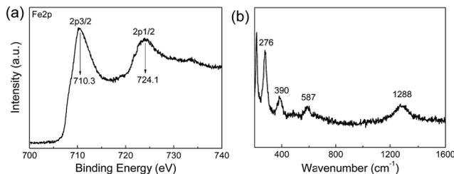
Fig. 4 Fe 2p core-level XPS spectrum (a) and Raman spectrum (b) of a JF/Fe<sub>3</sub>O<sub>4</sub> nanocomposite hydrogel prepared at a Fe<sup>2+</sup>/Fe<sup>3+</sup> concentration of 0.5 M.
