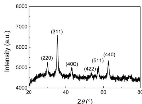
Fig. 3 X-ray diffraction pattern of the JF/Fe<sub>3</sub>O<sub>4</sub> nanocomposite hydrogel prepared at a Fe<sup>2+</sup>/Fe<sup>3+</sup> concentration of 0.5 M.
