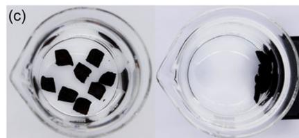
Fig. 6 (a) Magnetization curve of the JF/Fe<sub>3</sub>O<sub>4</sub> nanocomposite hydrogel prepared at a Fe<sup>2+</sup>/Fe<sup>3+</sup> concentration of 0.5 M (inset: enlarged magnetization curve); (b) saturation magnetization ( $M_s$ ) of JF/Fe<sub>3</sub>O<sub>4</sub> nanocomposite hydrogels as a function of Fe<sup>2+</sup>/Fe<sup>3+</sup> concentration; (c) photos demonstrating the attraction of JF/Fe<sub>3</sub>O<sub>4</sub> nanocomposite hydrogel specimens with a magnet.
