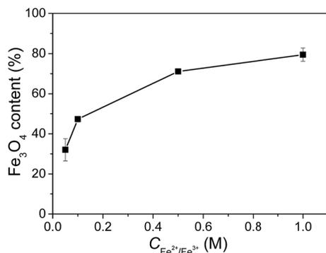
Fig. 5 Fe<sub>3</sub>O<sub>4</sub> contents in the JF/Fe<sub>3</sub>O<sub>4</sub> nanocomposite hydrogels prepared at different Fe<sup>2+</sup>/Fe<sup>3+</sup> concentrations.
