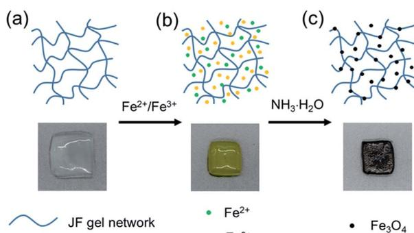
Fig. 1 Schematic representation and photos showing the preparation of JF/Fe<sub>3</sub>O<sub>4</sub> nanocomposite hydrogels. (a) An original JF gel, (b) the Fe<sup>2+</sup>/Fe<sup>3+</sup> loaded JF gel, and (c) the JF/Fe<sub>3</sub>O<sub>4</sub> nanocomposite hydrogel.
