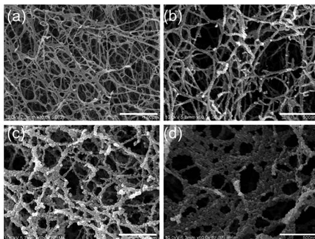
Fig. 2 SEM images of an original JF gel (a) and the JF/Fe<sub>3</sub>O<sub>4</sub> nanocomposite hydrogels prepared at the Fe<sup>2+</sup>/Fe<sup>3+</sup> concentrations of 0.1 M (b), 0.5 M (c) and 1.0 M (d).
