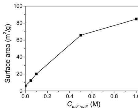
Fig. 7 Surface areas of the JF/Fe<sub>3</sub>O<sub>4</sub> nanocomposite hydrogels as a function of Fe<sup>2+</sup>/Fe<sup>3+</sup> concentration.
