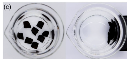
Fig. 6 (a) Magnetization curve of the JF/Fe 3 O 4 nanocomposite hydrogel prepared at a Fe 2+ /Fe 3+ concentration of 0.5 M (inset: enlarged magnetization curve); (b) saturation magnetization ( M_s ) of JF/Fe 3 O 4 nanocomposite hydrogels as a function of Fe 2+ /Fe 3+ concentration; (c) photos demonstrating the attraction of JF/Fe 3 O 4 nanocomposite hydrogel specimens with a magnet.
