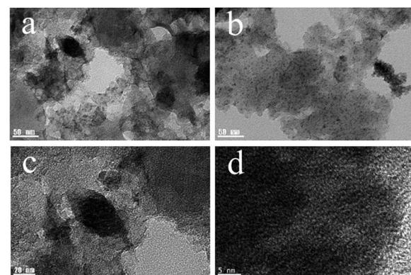
Fig. 5 TEM images of  $\gamma$ -Fe<sub>2</sub>O<sub>3</sub>/C.
