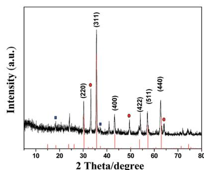
Fig. 1 XRD patterns of simulated  $\text{Fe}_2\text{O}_3$  and  $\gamma\text{-Fe}_2\text{O}_3/\text{C}$ .
