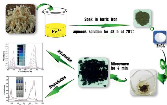
Scheme 1 Synthesis of  $\gamma\text{-Fe}_2\text{O}_3/\text{C}$ .
