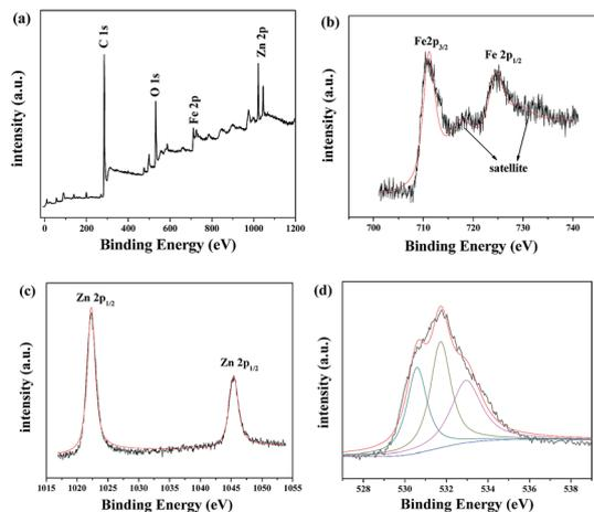
Fig. 2 XPS spectra of the as-prepared  $\gamma$ -Fe<sub>2</sub>O<sub>3</sub>/C: (a) survey spectrum; (b) high-resolution Fe 2p binding energy spectrum; (c) high-resolution Zn 2p binding energy spectrum; (d) high-resolution O 1s binding energy spectrum.
