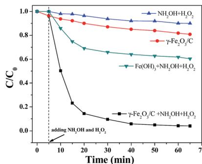
Fig. 8 Catalytic properties of different materials with MB ( $100 \text{ mg L}^{-1}$ ) at  $30^\circ\text{C}$  and  $\text{pH} = 7$  (the dosages of catalyst:  $10 \text{ mg}$ ;  $\text{C}_{\text{NH}_2\text{OH}}$ :  $10 \text{ mmol L}^{-1}$ ;  $\text{C}_{\text{H}_2\text{O}_2}$ :  $3 \text{ mol L}^{-1}$ ).
