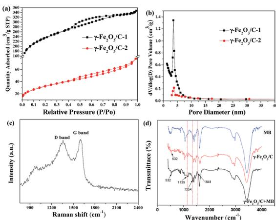
Fig. 3 (a) N<sub>2</sub> adsorption-desorption isotherm of  $\gamma$ -Fe<sub>2</sub>O<sub>3</sub>/C 1 and 2, and (b) the corresponding pore diameter distribution analysis (the FeCl<sub>3</sub> impregnation ratio of 1 and 2: 0.5 : 1, and 2 : 1; the carbonization time of 1 and 2: 4 min). (c) Raman spectrum of  $\gamma$ -Fe<sub>2</sub>O<sub>3</sub>/C. (d) FT-IR spectra of  $\gamma$ -Fe<sub>2</sub>O<sub>3</sub>/C with MB,  $\gamma$ -Fe<sub>2</sub>O<sub>3</sub>/C, and MB.
