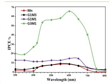
Fig. 8 Incident-photon-conversion efficiencies (IPCE%) of Mn<sub>3</sub>O<sub>4</sub>, G3M1, G1M1 and G1M3.
