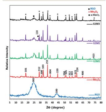
Fig. 1 XRD patterns of RGO, Mn<sub>3</sub>O<sub>4</sub>, G3M1, G1M1 and G1M3.
