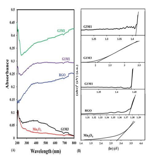
Fig. 4 UV-Vis absorption spectra of RGO, Mn<sub>3</sub>O<sub>4</sub>, G3M1, G1M1 and G1M3, and their corresponding plots of  $(\alpha h\nu)^2$  versus  $(h\nu)$  for energy bandgap  $(E_a)$  determination.
