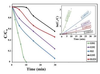
Fig. 10 Microwave degradation of MB dye by  $Mn_3O_4$ , RGO, G3M1, G1M1 and G1M3 nanocomposites: reaction conditions: (temp. = 373 K, catalyst weight 100 mg, dye conc. 20 ppm, 800 W, 2.45 GHz). Insets are the kinetic fits of MB degradation  $\emph{via}$  the as-synthesized nanocomposites.
