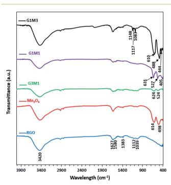
FTIR spectra of RGO, Mn<sub>3</sub>O<sub>4</sub>, G3M1, G1M1 and G1M3.
