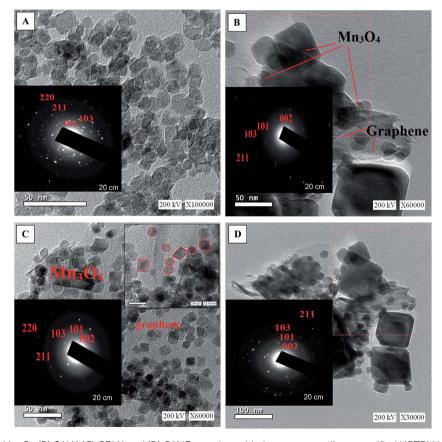
Fig. 2 TEM images of (A) Mn<sub>3</sub>O<sub>4</sub> (B) G1M1 (C) G3M1 and (D) G1M3 together with the corresponding magnified HRTEM images and SAED patterns, as insets.
