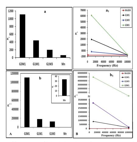
Fig. 13 The dielectric constant (a) and dielectric loss (b) of  $Mn_3O_4$ , G3M1, G1M1 and G1M3 and their counterparts (a<sub>1</sub>) and (b<sub>1</sub>) as a function of frequency change in the margin from 1.0 Hz to 100 kHz.
