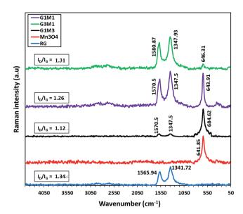
Fig. 5 Raman spectra of Mn<sub>3</sub>O<sub>4</sub>, G3M1, G1M1 and G1M3.
