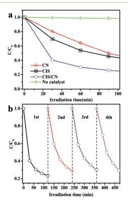
Fig. 4 (a) Photocatalytic degradation of TC in the presence of CIS, CN, CIS/CN and in the absence of photocatalyst and (b) cycling runs for the photodegradation of TC with CIS/CN.
