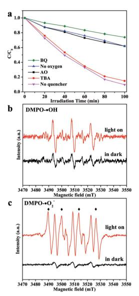
Fig. 5 (a) Trapping experiment of active species during the photocatalytic degradation of MO using CIS/CN under visible-light, and DMPO spin-trapping ESR spectra recorded with CIS/CN in aqueous dispersion for DMPO-OH (b) and in methanol dispersion for DMPO-'O<sub>2</sub>- (c)
