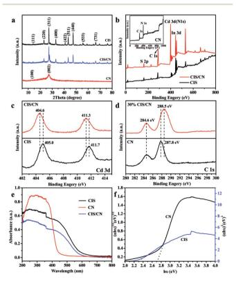
Fig. 2 (a) XRD patterns, (b) XPS survey spectra of CIS, CN (inset) and CIS/CN, (c and d) high-resolution XPS spectra of Cd 3d and C 1s, respectively, (e) UV-vis spectroscopy, and (f) plot of  $(\alpha h \nu)^{1/2}$  vs.  $h \nu$  for the band gap energy of CN and plot of  $(\alpha h \nu)^2$  vs.  $h \nu$  for the band gap energy of CIS.
