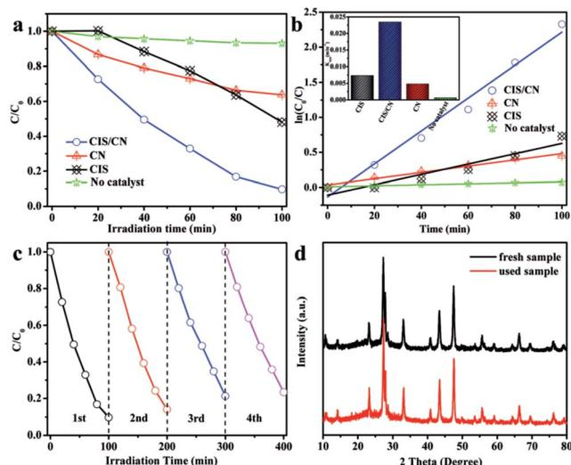
Fig. 3 (a) Photocatalytic degradation of MO and (b) kinetic fit and degradation rate constant  $k$  (inset in b) for the degradation of MO using CIS, CN, CIS/CN and in absence of photocatalyst, (c) cycling runs for the photodegradation of MO with CIS/CN, and (d) XRD patterns of the freshly prepared and used CIS/CN after four times cycling.
