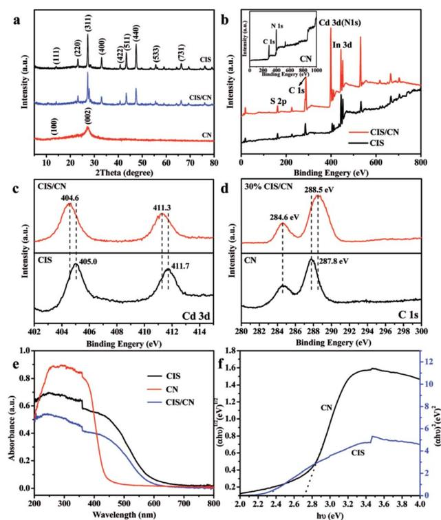
Fig. 2 (a) XRD patterns, (b) XPS survey spectra of CIS, CN (inset) and CIS/CN, (c and d) high-resolution XPS spectra of Cd 3d and C 1s, respectively, (e) UV-vis spectroscopy, and (f) plot of  $(\alpha h\nu)^2$  vs.  $h\nu$  for the band gap energy of CN and plot of  $(\alpha h\nu)^{1/2}$  vs.  $h\nu$  for the band gap energy of CIS.
