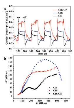
Fig. 8 (a) Transient photocurrent responses and (b) EIS Nyquist plots of CIS, CN and CIS/CN.
