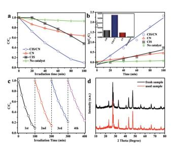
Fig. 3 (a) Photocatalytic degradation of MO and (b) kinetic fit and degradation rate constant k (inset in b) for the degradation of MO using CIS, CN, CIS/CN and in absence of photocatalyst, (c) cycling runs for the photodegradation of MO with CIS/CN, and (d) XRD patterns of the freshly prepared and used CIS/CN after four times cycling.
