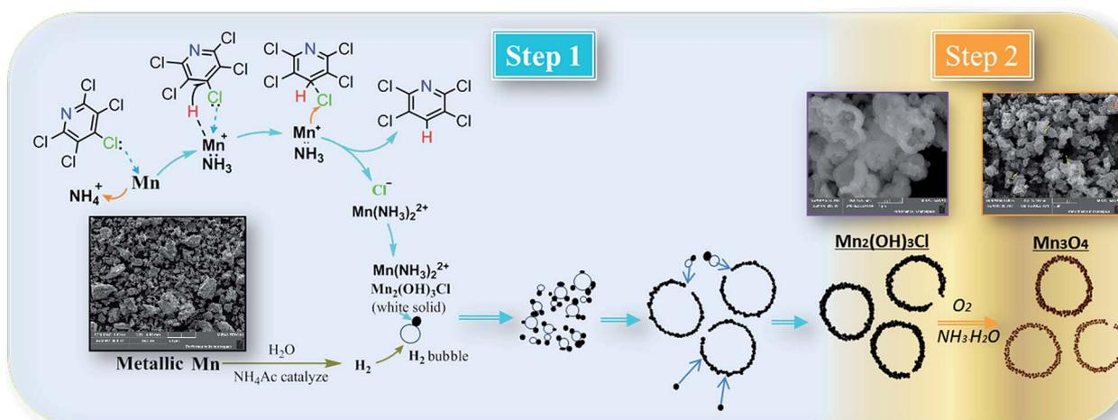
Scheme 1 Possible mechanism for hydrodechlorination reaction process and formation processes of hollow microspheres.
