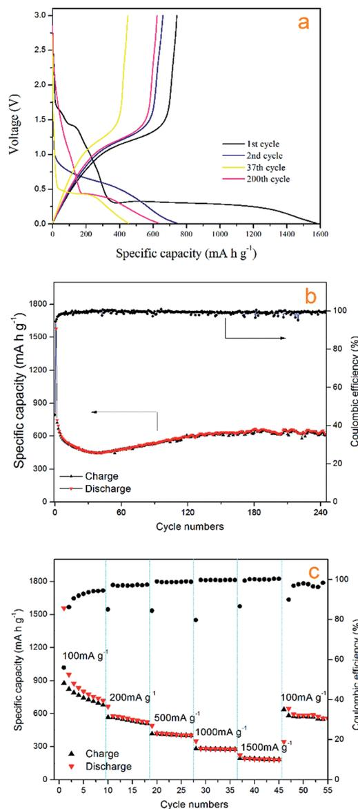
Fig. 7 (a) The 1<sup>st</sup>, 2<sup>nd</sup>, 37<sup>th</sup> and 200<sup>th</sup> voltage profiles of the  $\text{Mn}_3\text{O}_4$  electrode between 0.01 and 3.00 V at a current density of  $200 \text{ mA g}^{-1}$ . (b) Cycle performance and coulombic efficiency *versus* cycle number of  $\text{Mn}_3\text{O}_4$  hollow spheres at a current density of  $200 \text{ mA g}^{-1}$ . (c) Rate capabilities with increasing current density.
