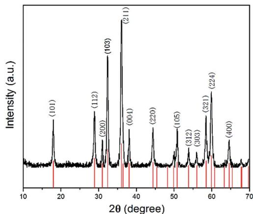
Fig. 1 XRD pattern of  $\text{Mn}_3\text{O}_4$  hollow microspheres.
