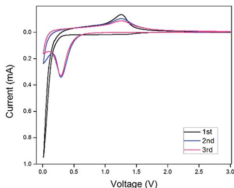
Fig. 6 Cyclic voltammetry (CV) curves of the 1<sup>st</sup>, 2<sup>nd</sup> and 3<sup>rd</sup> cycles for the  $\text{Mn}_3\text{O}_4$  hollow microspheres at a scan rate of  $0.40 \text{ mV s}^{-1}$  between 0.01 and 3.00 V.
