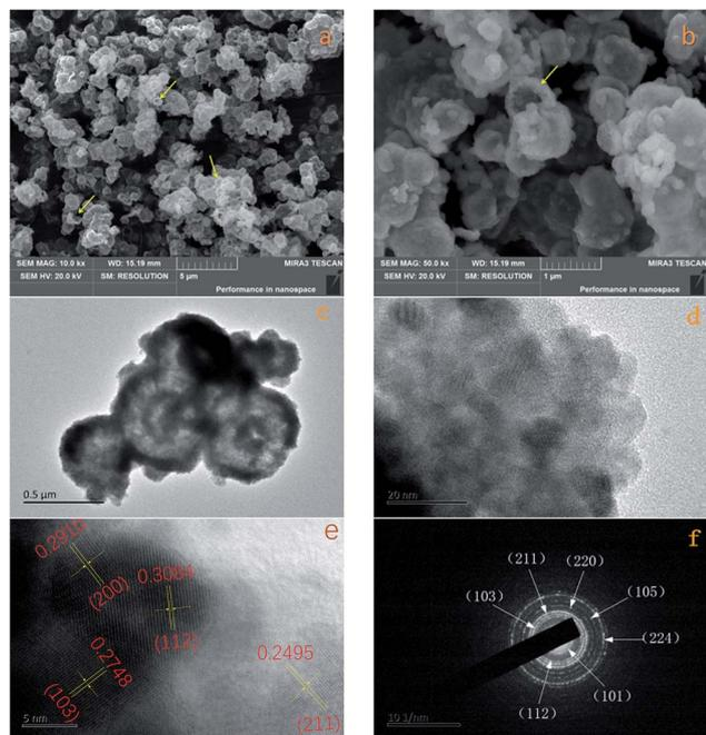
Fig. 2 (a) Representative FE-SEM images of  $\text{Mn}_3\text{O}_4$  and (b) FE-SEM image of partial enlarged detail (c) TEM image of  $\text{Mn}_3\text{O}_4$ ; (d) TEM image of partial enlarged detail; (e) HR-TEM image of partial enlarged detail; (f) SAED image of  $\text{Mn}_3\text{O}_4$ .
