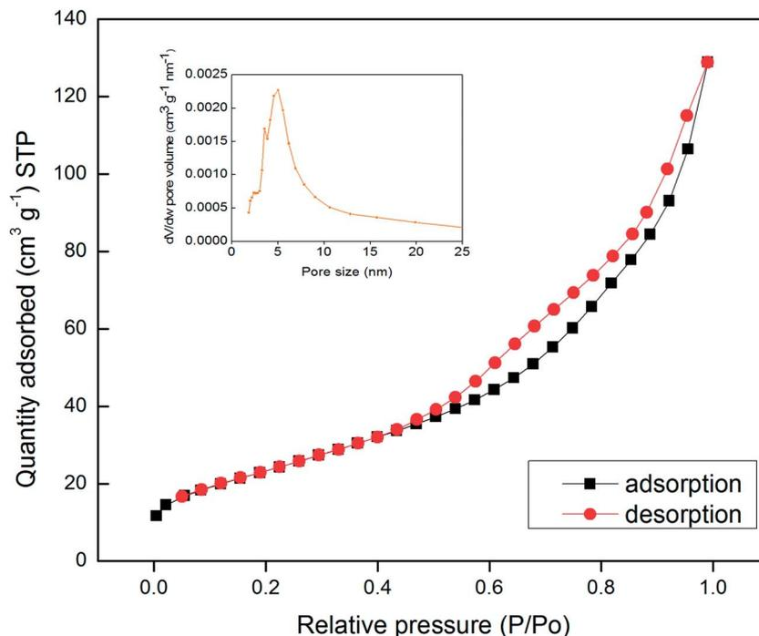
Fig. 3  $N_2$  adsorption isotherms and pore size distribution (insets) of  $Mn_3O_4$  hollow microspheres.
