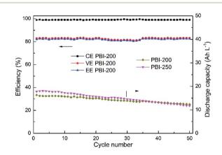
Cycling performance over 50 cycles of VFBs with the prepared PBI membranes at constant current density of 80 mA cm<sup>-2</sup>.
