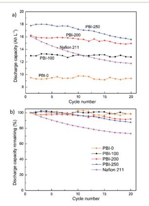
Fig. 8 (a) Discharge capacity and (b) discharge capacity retention of VFBs with the prepared PBI membranes and Nafion 211 at constant current density of 80 mA cm<sup>-2</sup>.
