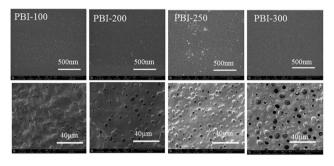
Fig. 2 SEM images of the top and the bottom surfaces of the asymmetric PBI membranes (top row: the top surfaces; bottom row: the bottom surfaces).
