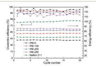
Fig. 7 Efficiencies of VFBs with the prepared PBI membranes and Nafion 211 at constant current density of 80 mA cm<sup>-2</sup>.
