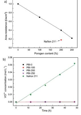
Fig. 5 (a) AR and (b) vanadium diffusion of the prepared PBI membranes and Nafion 211.
