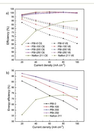
Fig. 6 Efficiencies of the VFBs assembled with the prepared PBI membranes and Nafion 211 under different current densities.
