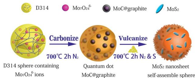
Fig. 1 Schematic representation showing synthesis of MoS<sub>2</sub>/C nanocomposite.
