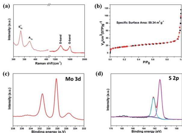
Fig. 3 (a) Raman spectra of MoS<sub>2</sub>/C, (b) N<sub>2</sub> adsorption/desorption isotherms of MoS<sub>2</sub>/C, (c) Mo 3d and (d) S 2p XPS spectra of the MoS<sub>2</sub> nanosheets.
