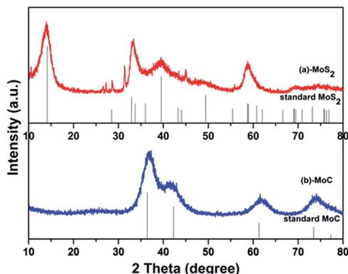
Fig. 2 XRD patterns of prepared (a) MoC/C nanocomposite and MoC standard, and (b) MoS<sub>2</sub>/C nanocomposite and MoS<sub>2</sub> standard.
