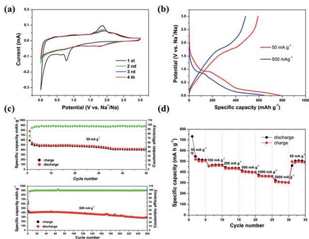
Fig. 5 Electrochemical performance of the MoS<sub>2</sub>/C nanocomposite: (a) CV curves at scan rate 0.1 mV s<sup>-1</sup>; (b) first galvanostatic discharge/charge profiles at current densities 50 and 500 mA g<sup>-1</sup>; (c) cycling performance and corresponding coulombic efficiency; and (d) rate capacity at different current densities.
