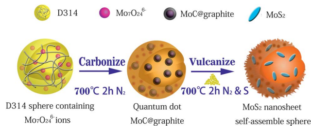
Fig. 1 Schematic representation showing synthesis of MoS 2 /C nanocomposite.
