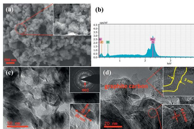
Fig. 4 MoS<sub>2</sub>/C nanocomposite characterized by (a) SEM image, (b) energy dispersive spectrum, (c) TEM images, and (d) HRTEM image.
