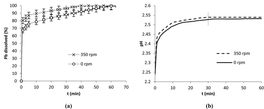
Fig. 5 Dissolution of Pb in  $\text{HNO}_3$  (a) and the evolution of pH (b) in the presence and absence of stirring. Operation conditions: 0.1 g Pb, 25 °C,  $V = 250$  mL,  $\text{HNO}_3$  at 5 mM.
