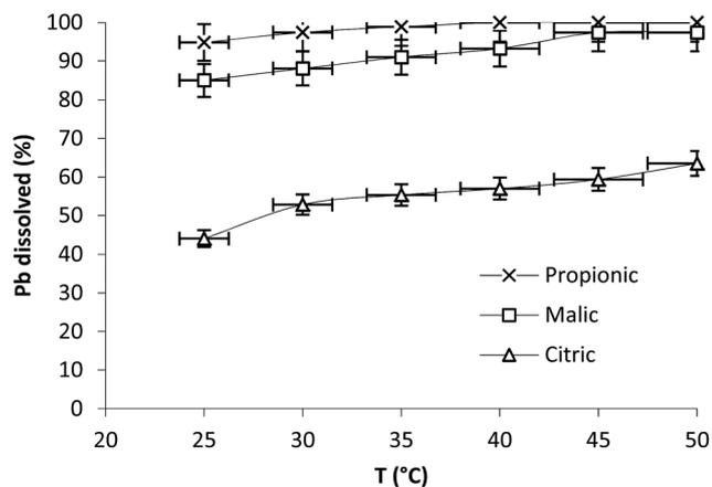
Fig. 3 Effect of temperature on Pb dissolution with the three organic acids after 20 min. Operation conditions: 0.1 g Pb,  $t = 20$  min, 350 rpm,  $V = 250$  mL,  $C_{acid} = 5$  mM.
