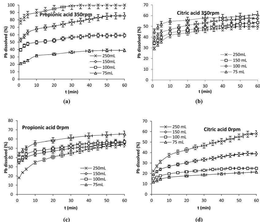
Fig. 6 Effect of the hydrodynamic conditions on Pb dissolution with propionic and citric acids. (a and b) 350 rpm, (c and d) 0 rpm. Operation conditions: 0.1 g Pb, 25 °C,  $n_{\text{acid}} = 1.25 \times 10^{-3}$  mol.
