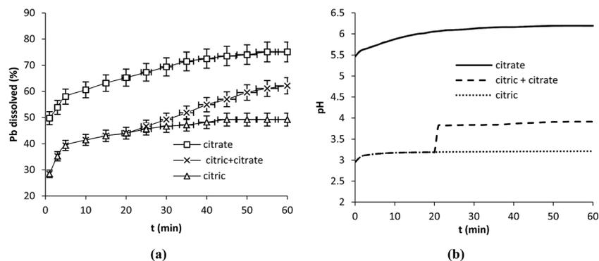
Fig. 4 Effect of the addition of citrate ligand on Pb dissolution (a) and on the evolution of pH (b) during Pb dissolution. Operation conditions: 0.1 g Pb, 25 °C, 350 rpm,  $V = 250$  mL,  $C_{\text{acid}} = 5$  mM,  $C_{\text{citrate}} = 5$  mM.
