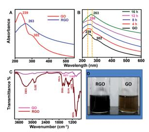
Fig. 1 (A) UV/Vis spectrum of GO and sRGO (B) the kinetics data showing the transformation of GO to sRGO with respect to time (C) ATR-IR spectrum of GO and sRGO (D) photographic images of GO (right) and sRGO (left). Traces are shifted vertically for clarity.
