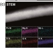
Fig. 2 (a) SEM image of PMN-PT NWs synthesized by a hydrothermal method. (b) TEM image of PMN-PT NWs. The Left-top inset is a HRTEM image of a single NW showing that lattice fringes of the (110) plane and the right-bottom image shows the SAED pattern when the electron beam is coherent along the [001] plane. (c) STEM image and EDS mapping of a PMN-PT NW.
