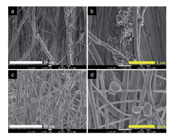
Fig. 1 Morphology of (a and b) MgO/mNAF and (c and d) POM/mANF nanofibre composites used as outer layers of nanofibrous protective materials.
