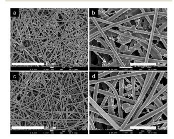
Fig. 4 Morphology of (a and b) [I]MgO/PANF and (c and d) [I]POM/PANF nanofibre composites used as inner layers of nanofibrous protective materials.
