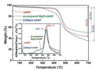
Fig. 2 Differential thermal analysis (inset) and thermal gravimetric analysis of neat mANF, as-prepared MqO/mANF, and [O]MqO/mANF.
