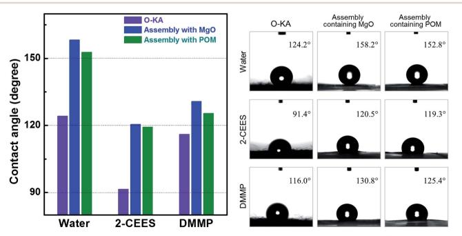
Fig. 6 Amphiphobic surface behavior of the outer layer of permeable protective clothing used by the Korean Army (O-KA), and assemblies containing MgO and POM as nanofibrous protective materials against CWA simulants 2-CEES and DMMP.
