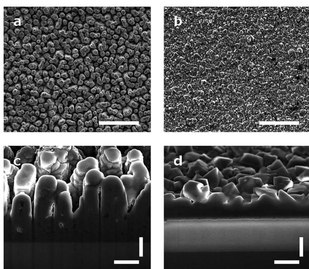
Fig. 2 (a and b) Top view of DCNT (1  $\mu\text{m}$  CNT length) and of flat diamond control sample respectively. Scale bars, 4  $\mu\text{m}$  (c and d) cross section of DCNT sample (1  $\mu\text{m}$  CNT length) and flat diamond control sample respectively. Scale bars, 0.5  $\mu\text{m}$ .
