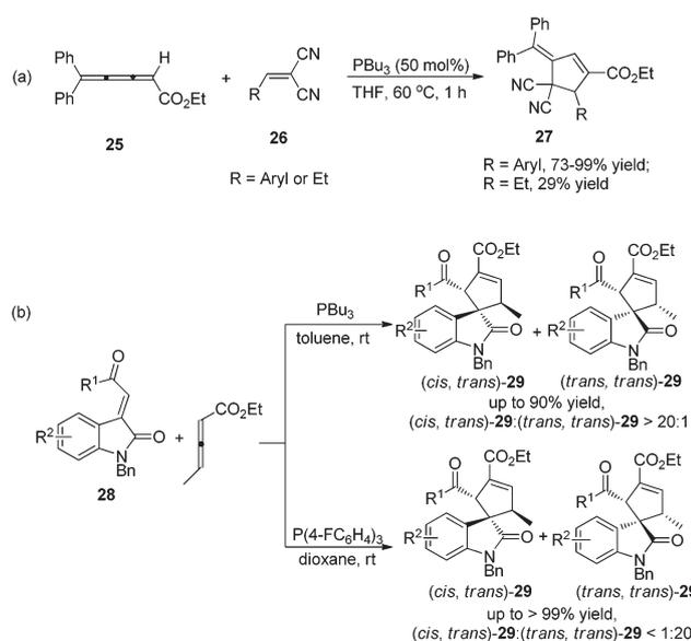
**Scheme 8** Synthesis of polysubstituted cyclopentenes and spirocyclic products through Lu's [3 + 2] cycloaddition developed by Shi's group.
