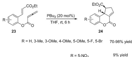
Scheme 7 Synthesis of dihydrocoumarins through intramolecular Lu's [3 + 2] cycloaddition.
