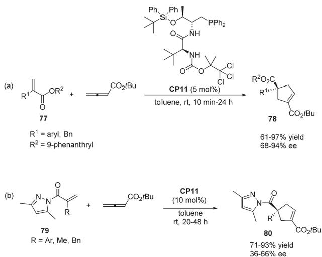
**Scheme 22** The catalytic asymmetric Lu's [3 + 2] cycloadditions developed by Lu's group.
