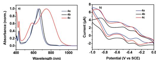
**Fig. 3** (a) Optical absorption spectra of **4a–c** in solution with a concentration of  $2 \times 10^{-5}$  M. (b) Cyclic voltammograms of **4a–c** ( $10^{-3}$  mol L $^{-1}$ ) with 0.1 M Bu $_4$ NPF $_6$  in chloroform solution and a scan rate of 50 mV s $^{-1}$  (vs. SCE).
