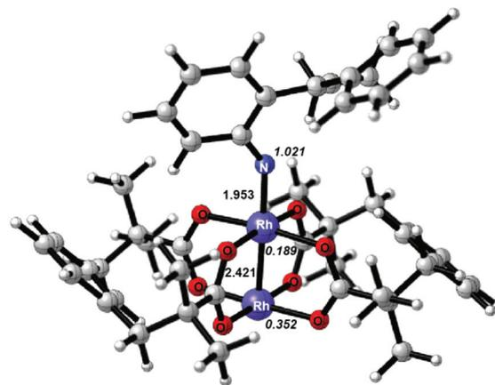
**Fig. 1** Optimized structure at the BS1 level for the  $\text{Rh}_2$ -nitrene <sup>3</sup>**IN2**; key bond lengths (Å) and spin densities on nitrogen and rhodium atoms (in italics) are indicated.
