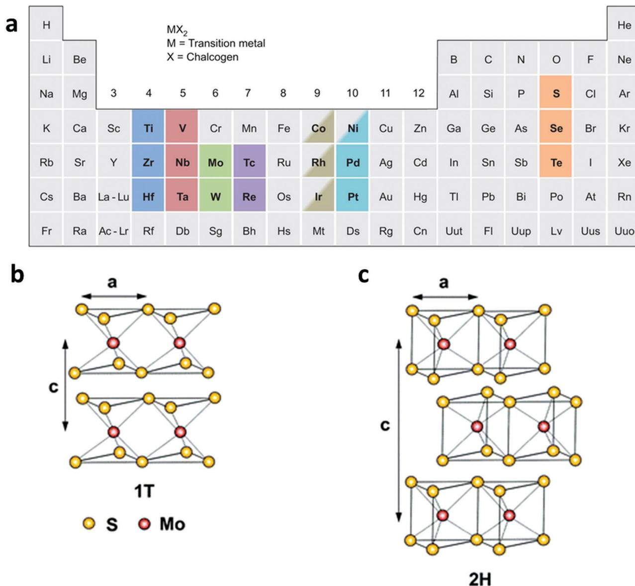
Fig. 1 (a) Various kinds of TMD nanomaterials, reproduced with permission from ref. 20. Copyright 2013 Nature Publishing Group. Schematic illustration of (b) the 1T-type and (c) the 2H-type structure of  $MoS_2$ . Reproduced with permission from ref. 8. Copyright 2013 Royal Society of Chemistry.
