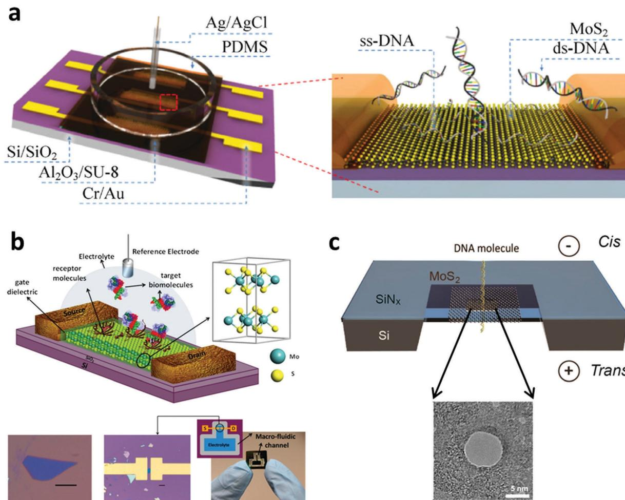
Fig. 4 (a) Schematic illustration of MoS<sub>2</sub>-based FET. Reproduced with permission from ref. 130. Copyright 2015 Springer. (b) Schematic diagram of the MoS<sub>2</sub>-based FET biosensor. Reproduced with permission from ref. 132. Copyright 2014 American Chemical Society. (c) Schematic illustration of a MoS<sub>2</sub> nanopore membrane for DNA translocation. Reproduced with permission from ref. 139. Copyright 2014 American Chemical Society.
