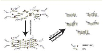
Scheme 1 Schematic illustration of pTh-Pdot synthesis
