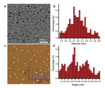
Fig. 1 (a) High-resolution TEM image of pTh-Pdots. (b) Diameter distribution (n = 200). (c) AFM image of pTh-Pdots. Inset shows the height profile along the indicated line. (d) Height distribution (n = 200).
