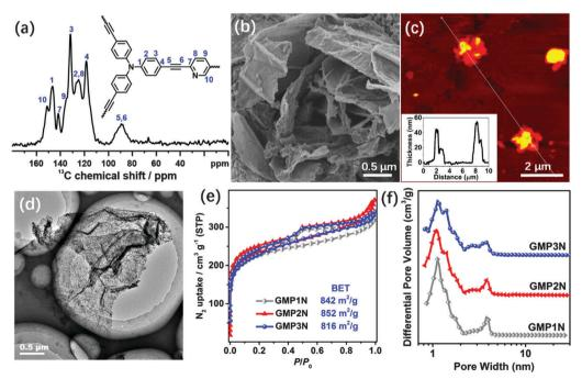
Fig. 1 Structure and morphological characterization of graphene-based conjugated microporous polymers (GMPs). (a) The <sup>13</sup>C CP/MAS NMR spectrum of GMP1N and its peak assignments. (b) SEM, (c) AFM (inset: thickness analyses along the marked line), and (d) TEM images of GMP2N. (e) Nitrogen adsorption/desorption isotherms and (f) pore size distribution profiles of GMPs.
