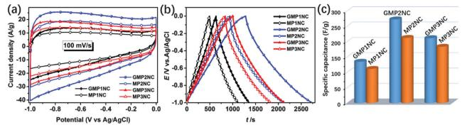
Fig. 4 Electrochemical characterization of the carbon materials derived from GMPs and graphene-free MPs in three-electrode systems using 6 M aqueous KOH solution as electrolyte. (a) CV curves at a scan rate of 100 mV  $s^{-1}$ . (b) Galvanostatic charge/discharge (GCD) curves and (c) the corresponding gravimetric capacitances at a current density of 0.2 A q<sup>-1</sup>.
