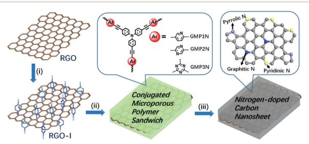
Scheme 1 Preparation of graphene-based conjugated microporous polymer sandwiches and related nitrogen-doped microporous carbon nanosheets. (i) Sodium dodecylbenzenesulfonate, 4-iodophenyl diazonium salt, 0 °C (2 h) to RT (4 h); (ii) building blocks: tris(4-ethynylphenyl)amine and 2,5-dibromopyridine, or 2,5-dibromopyrazine, or 2,4,6-trichloro-1,3,5-triazine, argon, Pd(PPh<sub>3</sub>)<sub>4</sub>, CuI, Et<sub>3</sub>N, DMF, 120 °C, 3 days; (iii) argon, RT to 800 °C, 10 °C min<sup>-1</sup>, 2 h.
