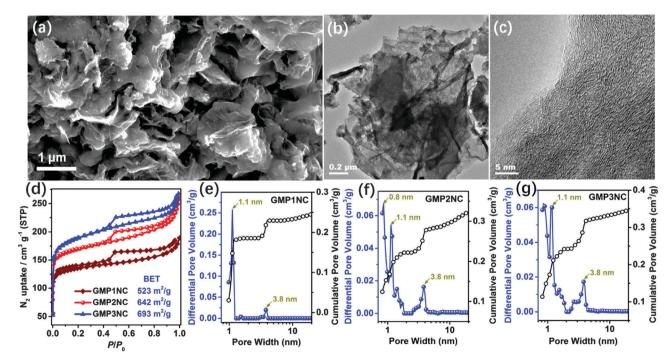
Fig. 2 Morphology and porosity of GMP-derived carbon nanosheets. (a) SEM, (b) TEM and (c) HRTEM images of GMP2N. (d) Nitrogen adsorption/desorption isotherms and (e-g) NLDFT-based pore size distribution and cumulated pore volume of GMP-derived carbon nanosheets
