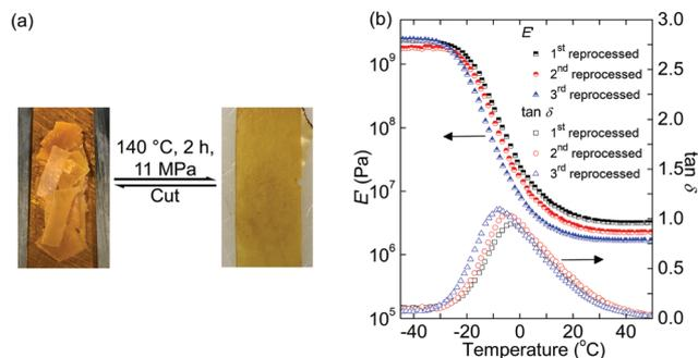
**Fig. 1** (a) Photograph of a PPGDC-TAEA PHU sample before and after reprocessing. (b) Dynamic mechanical responses of PPGDC-TAEA PHU networks,  $E'$  (half-open symbols) and  $\tan \delta$  (open symbols) as a function of temperature for the 1<sup>st</sup> reprocessed (squares), 2<sup>nd</sup> reprocessed (circles) and 3<sup>rd</sup> reprocessed (triangles) samples.
