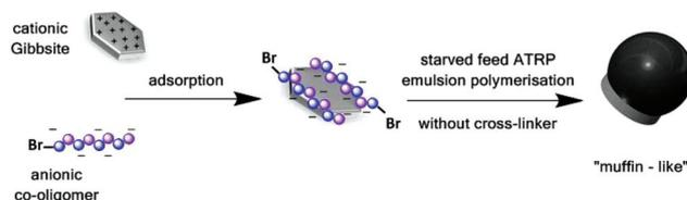
**Scheme 1** Schematic illustration of ATRP-based synthesis of polymer–Gibbsite nanocomposites using an anionic co-oligomer as a stabiliser and macroinitiator.
