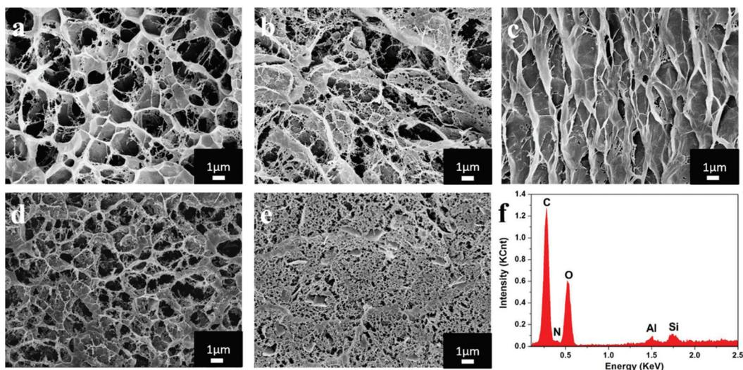
**Fig. 3** SEM images of hydrogels with a weight ratio of (a) chitosan : cellulose = 9 : 1, 5% REC; (b) chitosan : cellulose = 3 : 1, 5% REC; (c) chitosan : cellulose = 3 : 1, 10% REC; (d) chitosan : cellulose = 1 : 1, 5% REC; (e) chitosan : cellulose = 1 : 9, 5% REC and (f) EDS spectrum of sample b.
