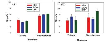
Fig. 2 Comparison of the swellability (*Q*) for toluene and fluorobenzene derived HCPs (prepared using 2 equivalents of FDA) against the three simulants triethylamine (NEt<sub>3</sub>), ethyl acetate (EtOAc), and dimethylformamide (DMF) using (a) Method 1 and (b) Method 2.
