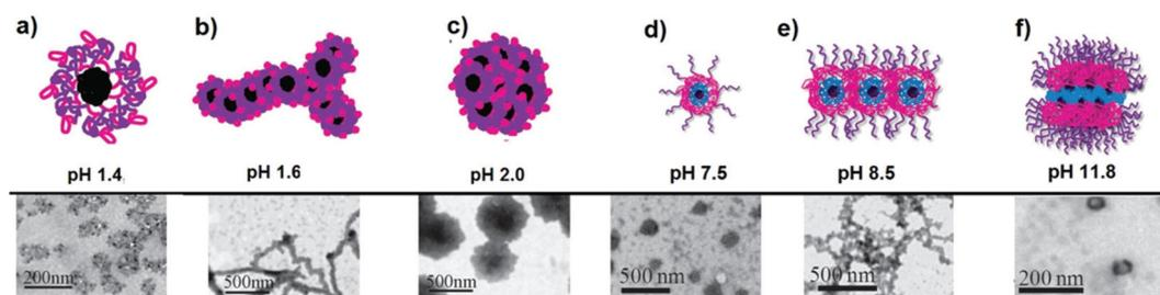
**Fig. 10** TEM images of the PS<sub>n</sub>-core-(P2VP-*b*-PAAc)<sub>n</sub> star conformation and the corresponding self-assemblies aqueous solution at: (a) pH 1.4 unimolecular micelle, (b) pH 1.6 worm-like micelle, (c) pH 2.0 multicore micelle, (d) pH 7.5 unimolecular micelle, (e) pH 8.5 unimolecular micelle association towards network-like assemblies, and (f) pH 11.8 multi-compartment multi-molecular micelle (Copyright 2011, The Royal Society of Chemistry, modified from ref. 202).
