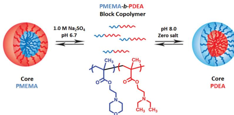
Fig. 7 Schematic representation of the formation of micelles and reverse micelles for a schizophrenic PMEMA-*b*-PDEA diblock copolymer in aqueous solution.<sup>151</sup>
