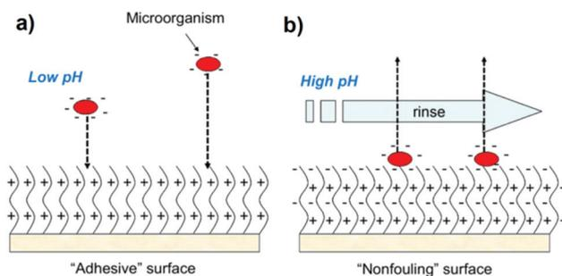
**Fig. 24** A surface switching from fouling to non-fouling in response to pH change: (a) in low pH solutions where the surface bears a moderately positive charge, favoring the attachment of bacteria cells, and (b) in neutral or higher pH solutions where the surface becomes non-fouling, releasing the bacteria cells (Copyright 2010, Elsevier Ltd, reprinted from ref. 239).
