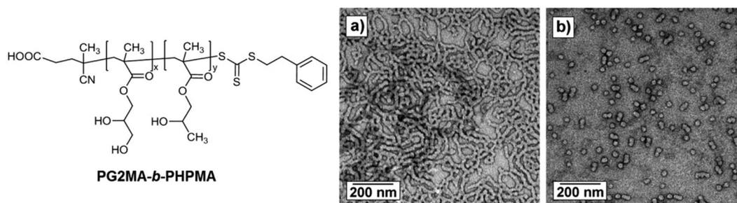
**Fig. 8** TEM images obtained on addition of NaOH followed by dilution of a 10% w/w aqueous dispersion of a PG2MA<sub>56</sub>-*b*-PHPMA<sub>155</sub> diblock copolymer prepared using the carboxylic acid functionalized PETTC RAFT agent: (a) pH 3.5 (initial worms); and (b) pH 6.0 (spheres) (Copyright 2015, Wiley-VCH Verlag GmbH & Co. KGaA, Weinheim, modified from ref. 134).
