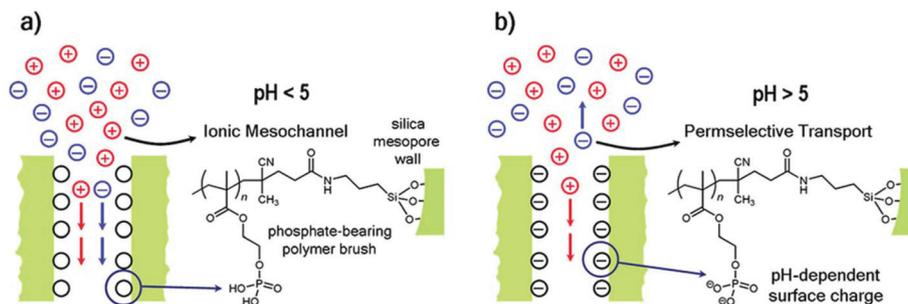
**Fig. 22** Schematic depiction of the ionic transport processes taking place in the hybrid polymer–inorganic interfacial assembly at different pH values: (a) pH < 5, ionic mesochannel (no exclusion of ionic species) and (b) pH > 5, permselective transport of cations (Copyright 2012, The American Chemical Society, reprinted from ref. 247).
