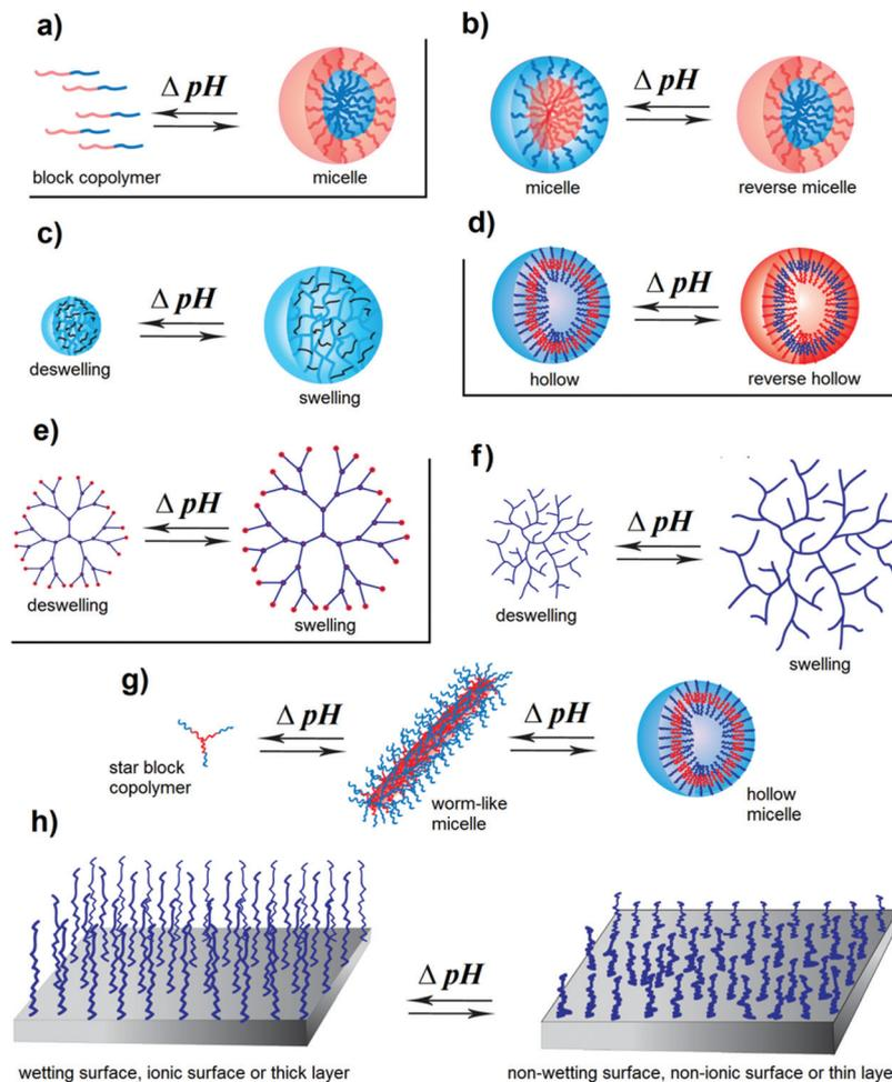
**Fig. 1** pH-Responsive polymers of different architectures: (a) unimer–micelle, (b) micelle–reverse micelle, (c) nanogels or microgels, (d) hollow–reverse hollow, (e) dendrimer, (f) hyper-branched, (g) micelle morphology changes (from worm-like to hollow), and (h) polymer brushes.
