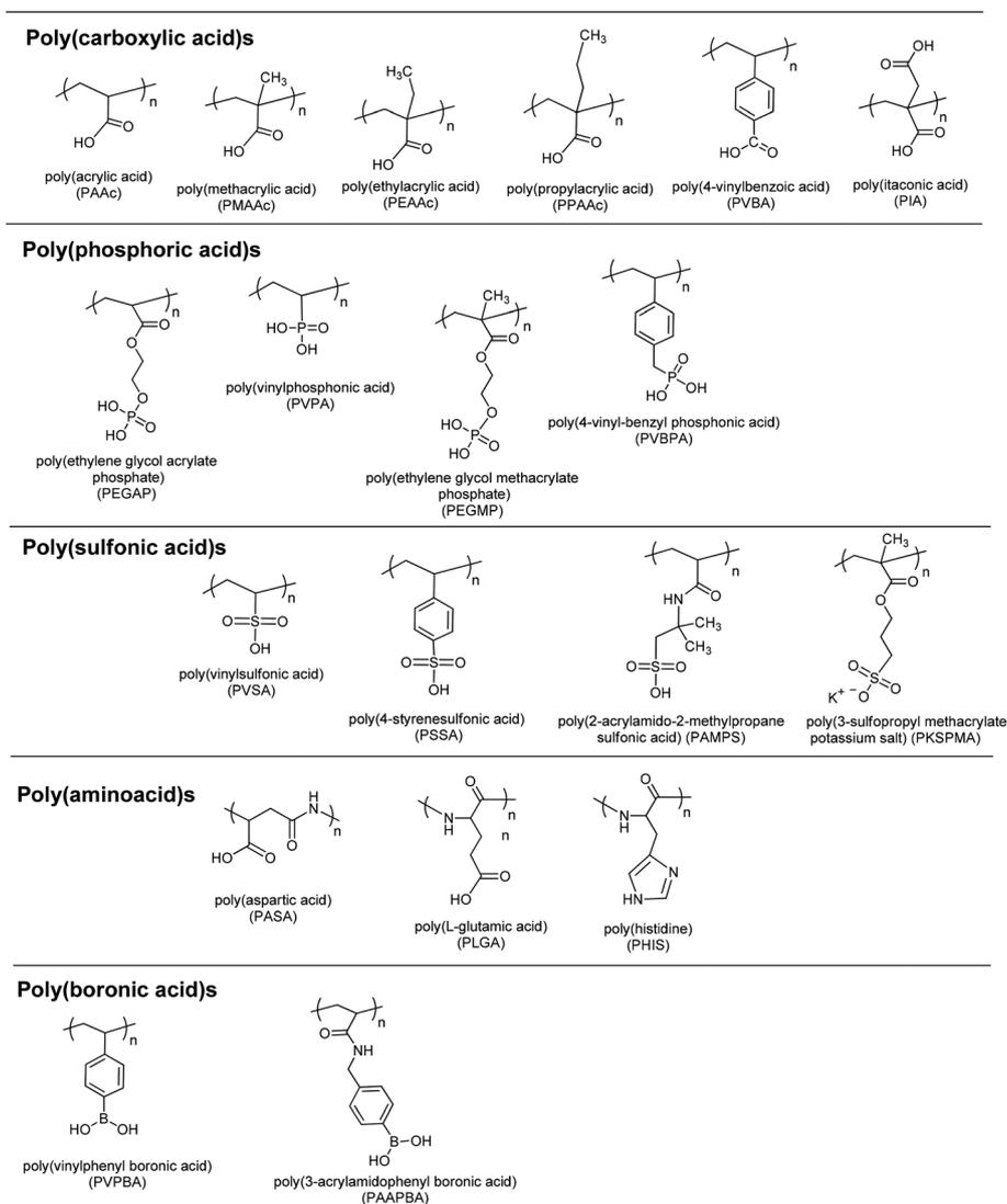
Fig. 2 Chemical structures of pH-responsive acidic polymers.
