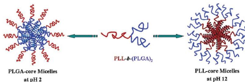
**Fig. 11** pH-Induced micellisation of PLL-*b*-(PLGA)<sub>2</sub> associated with coil-to-helix transitions (Copyright 2008, The American Chemical Society, reprinted from ref. 205).
