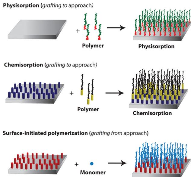
**Fig. 15** Synthetic strategies for the preparation of polymer brushes: (a) physisorption of diblock copolymers (grafting to), (b) chemisorption (grafting to) and (c) polymer brushes grown via surface-initiated polymerization (grafting from).
