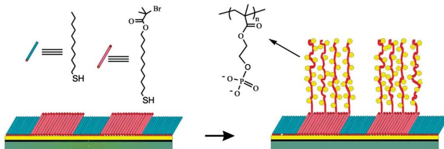
**Fig. 23** Procedure for patterned polymer brush formation on gold substrates. Polymer brush growth from initiator modified areas (Copyright 2005, The Royal Society of Chemistry, modified from ref. 392).
