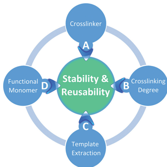
Fig. 1 The four main factors affecting the stability and reusability of molecularly imprinted polymers.
