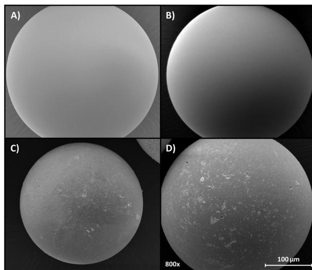
Fig. 6 Panel A shows a typical SEM image of freshly prepared IPs. Panel B shows a typical SEM image of IP1, IP3 and IP5 microspheres after the 100<sup>th</sup> cycle using the extraction method E2. Panels C and D reveal the deterioration of IP1 and IP5 after the 100<sup>th</sup> cycle using the extraction method E6, respectively. See Table 2 for the regeneration methods.
