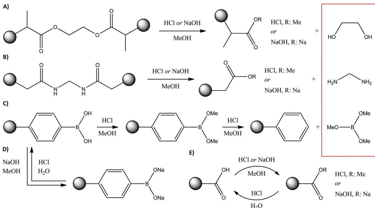
**Fig. 10** Degradation schemes of EDMA (A), BMA (B) crosslinked polymers, and esterification of acid based functional monomers *via* hydrolysis in methanol (C–E). The resulting esters or sodium salts remain part of the polymer network whilst ethylene glycol (A), methylenediamine (B) and trimethyl borate (C) leach out from the adsorbents (see in the box). The elimination by-products were isolated and their characterisation can be found in the ESI.†
