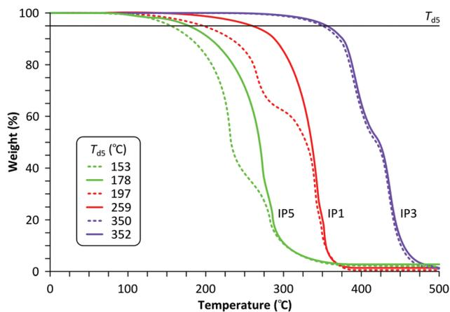
Fig. 5 TGA profiles and 5% decomposition temperature values ( $T_{d5}$ ) for BMA, EDMA and DVB crosslinked IP5, IP1 and IP3, respectively. Solid and dotted lines show the thermal stability after the 1<sup>st</sup> and 100<sup>th</sup> adsorption–regeneration cycle using E6, respectively.
