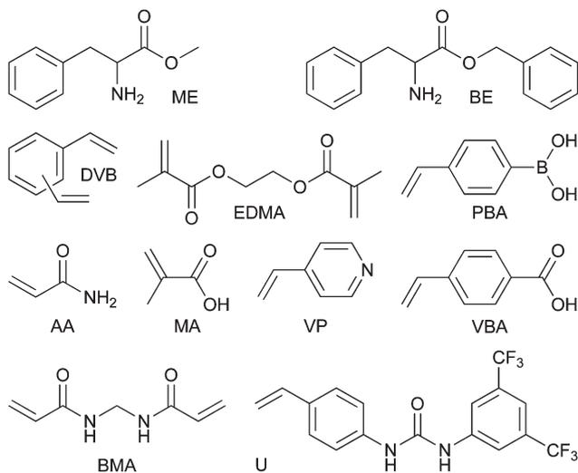
**Fig. 2** The L-phenylalanine methyl ester (ME) and benzyl ester (BE) were used as template and dummy template in this study. Ethylene glycol dimethacrylate (EDMA), divinylbenzene (DVB) and *N,N'*-methylenebis(acrylamide) (BMA) were employed as cross-linkers whilst methacrylic acid (MA), acrylamide (AA), 1-(4-vinylphenyl)-3-(3,5-bis(trifluoromethyl)phenyl)urea (U), 4-vinylpyridine (VP), 4-vinylphenylboronic acid (PBA) and 4-vinylbenzoic acid (VBA) were used as functional monomers.
