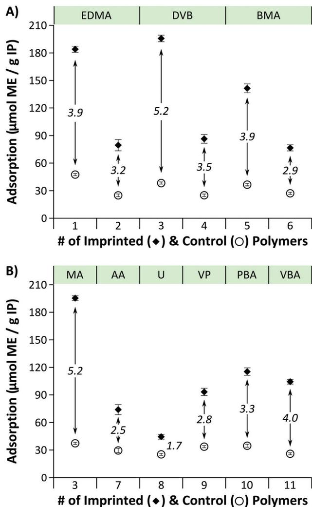
**Fig. 3** Initial adsorption of L-phenylalanine methyl ester (ME). Panel (A) includes IP1–IP6 imprinted and control polymers demonstrating the effect of crosslinker and crosslinking degree on adsorption. Panel (B) includes IP3, IP7–IP11 imprinted and control polymers showing the effect of functional monomer on adsorption. See Table 1 for the polymer compositions. Imprinting factors† are shown in italics.
