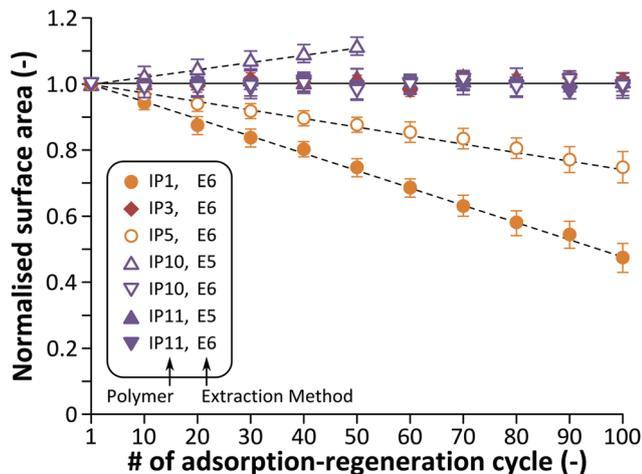
**Fig. 7** Normalised surface area obtained by Brunauer–Emmett–Teller (BET) analysis. Using the extraction method E6 the surface area for IP1 and IP5 monotonously decreases while for IP3, IP10 and IP11 remains virtually constant over time. On the other hand, the surface area increases for IP10 when the extraction method E5 is employed. See Table S2† in the ESI for the absolute surface area values.
