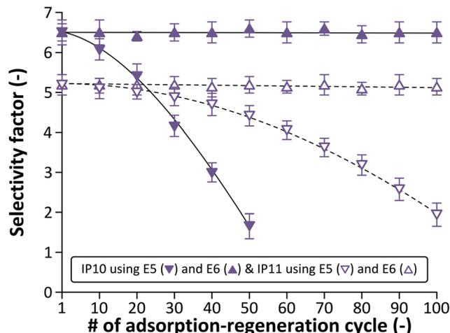
**Fig. 9** Selectivity factors for boronic acid (IP10) and carboxylic acid (IP11) based polymers using extraction methods E5 and E6. The results demonstrate that an acid wash enables maintaining the initial selectivity of the polymers.
