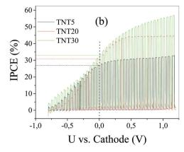
Fig. 6 Linear sweep voltammetry under chopped illumination of light intensity of 4 mW cm<sup>-2</sup> recorded at 5 mV s<sup>-1</sup> in 0.5 M Na<sub>2</sub>SO<sub>4</sub> vs. cathode (a), corresponding IPCE at the potential window from -0.8 V to 1.2 V vs. cathode. Dashed line denotes the IPCE at 0 V vs. cathode (b).
