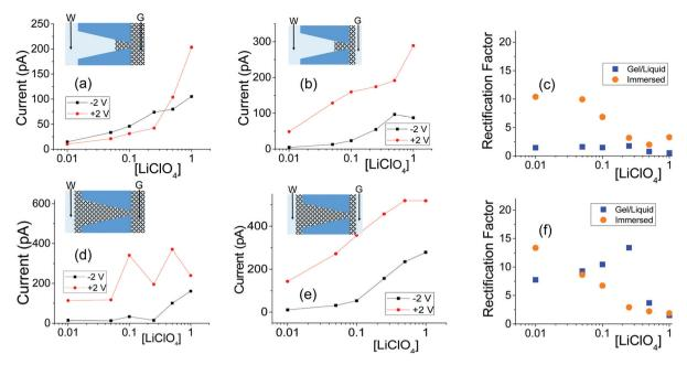
Fig. 6 (a, b) Recordings with a single conical nanopore with opening diameters of 515 nm (base) and 16 nm (tip); this pore was subjected to onesided drop cast of PMMA gel doped with 100 mM LiClO<sub>4</sub> (d, e) Measurements from another conical nanopore (1080 nm (base) and 18 nm (tip)), filled with PMMA gel. The base side was initially exposed to liquid electrolyte for the GLI test. Another set of data obtained with independently prepared pores in shown in Fig. S7.†
