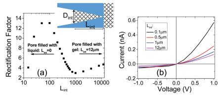
Fig. 7 (a) Scheme of a nanopore system subjected to numerical modeling. The pore considered had opening diameters of 25 nm and 500 nm; the pore length was 12  $\mu$ m. (b) Modeled I-V curves for four different values of  $L_{int}$ .
