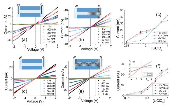
Fig. 2 (a-c) Ion current through a 790 nm in diameter cylindrical pore subjected to one-sided casting of undoped PMMA. (d-f) Experiments with a 640 nm pore after it had been filled with PMMA gel doped with 100 mM LiClO<sub>4</sub> (drop-casting had been performed on both sides of the membrane). Insets show state of the pore during the I-V scan. Inset on 3f shows I-V measurements of gel-only case and the immersed sample (100 mM LiClO<sub>4</sub>/PC).
