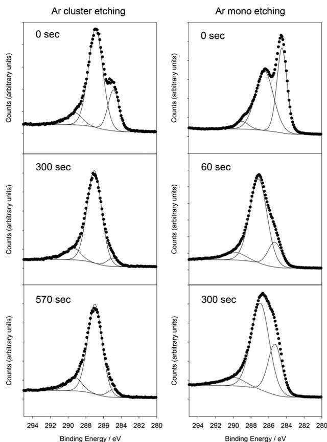
**Fig. 2** X-ray photoelectron spectra of the C 1s region of GCN film on glass. Data was fitted with three Gaussian-Lorentzian components as described in the text. Etching using monoatomic or clusters of Ar ions was used in an attempt to remove the graphitic carbon contamination. Spectra taken after various etching times using the different sources are shown. Mono Ar etching causes significant changes to the spectrum with extended etching, whereas cluster Ar etching does not.
