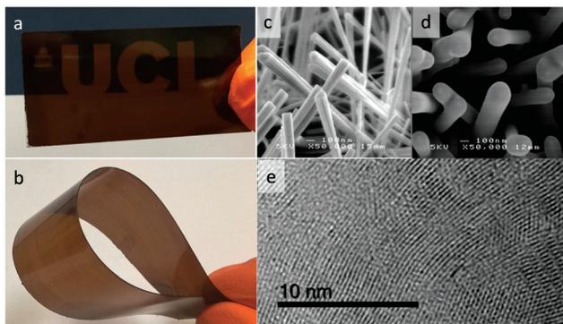
**Fig. 1** (a) GCN film deposited on glass. (b) GCN film deposited on acetate plastic. (c) SEM image of uncoated  $\text{WO}_3$  nanorods. (d) SEM image of  $\text{WO}_3$  nanorods coated with GCN (e) TEM image of GCN film coated directly onto a holey carbon grid, showing lattice fringes.
